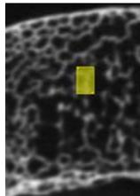
Figure 5. Selection of a bone-air interface for HMH thresholding in a micro-CT scan
