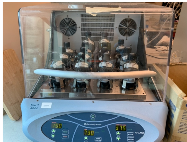
Figure 4-3: Anaerobic digestion batch test setup for liquid phase
