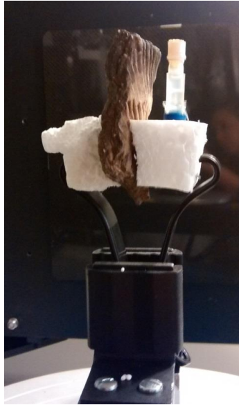
Figure 5.4: Secondary (cellphone) clamp with EPF. A water phantom is included in this scan. Water phantoms were used to run calibrated scans (see Section 6.2.4). They were created by placing distilled water in a clear plastic tube with caps on each end and mounted by creating a hole in the EPF next to the ceramic specimens.
