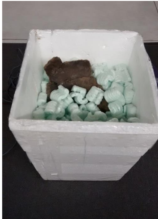
Figure 5.5: Ceramic mounted in EPF box surrounded by EPF peanuts.
