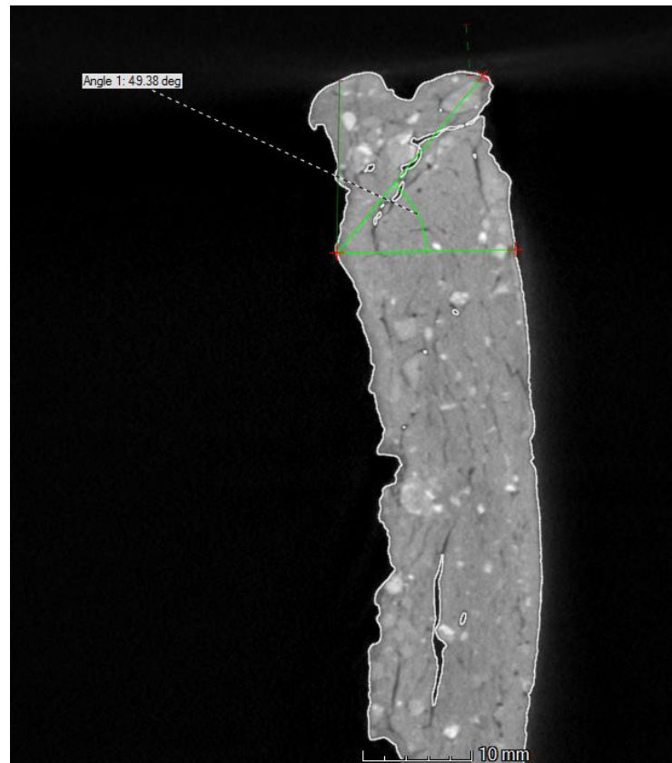
Figure 6.27: Example of a vessel (Specimen 100) with voids running parallel to vessel walls, but angled where the added section joins near the rim of the vessel. The void measured runs at a 49 degree angle then curves to run perpendicular to the vessel walls as it meets the interior wall.
