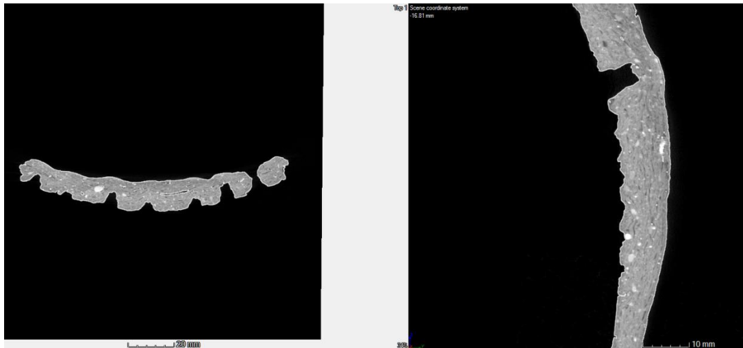
Figure 6.63: Specimen 040 - a round tool with a tip that appears blunt in the slice through the Z plane and bifurcated in the slice through the X plane.
