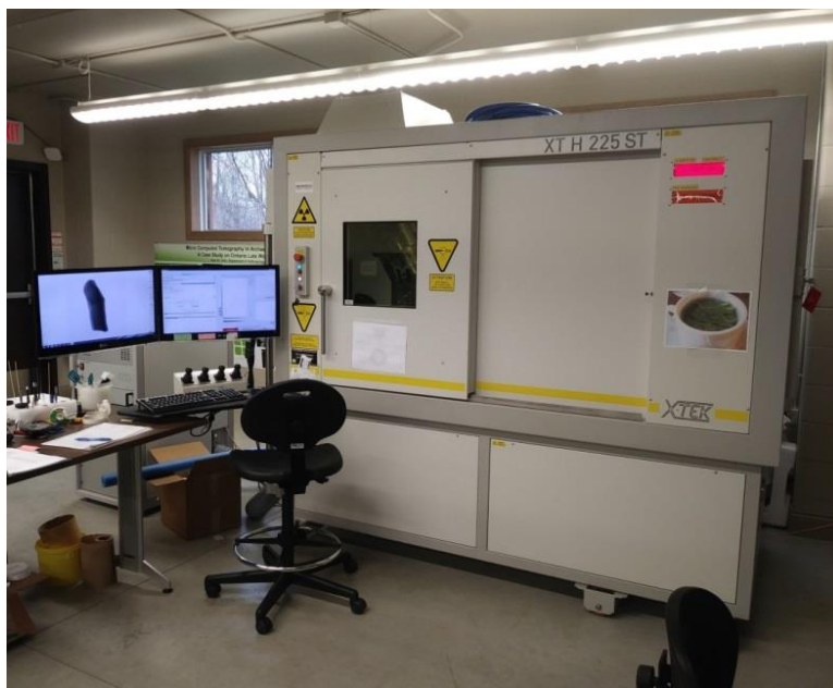
Figure 5.1: The scanner at the Museum of Ontario Archaeology operated by Western University, showing the chamber from the exterior with the door closed and the two acquisition computer screens to the left.
