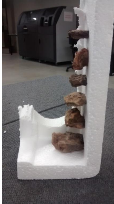
Figure 5.6: A stacked mounting method used to scan multiple small specimens at once, in the case scanning multiple clay lumps.
