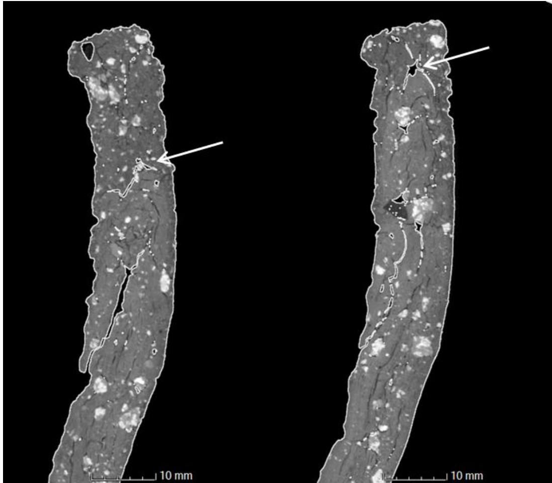
Figure 6.31: A rim (Specimen 050) that has been folded and then clay added on top. The scanned cross section at the left is through the castellation on the vessel. There is more clay added to create the castellation in this case. The joining void where clay has been added is indicated by arrows. Note also the difference in density in the clay above and below the fold; the clay above the fold appears as darker, indicating it has a lower density than clay below the fold.
