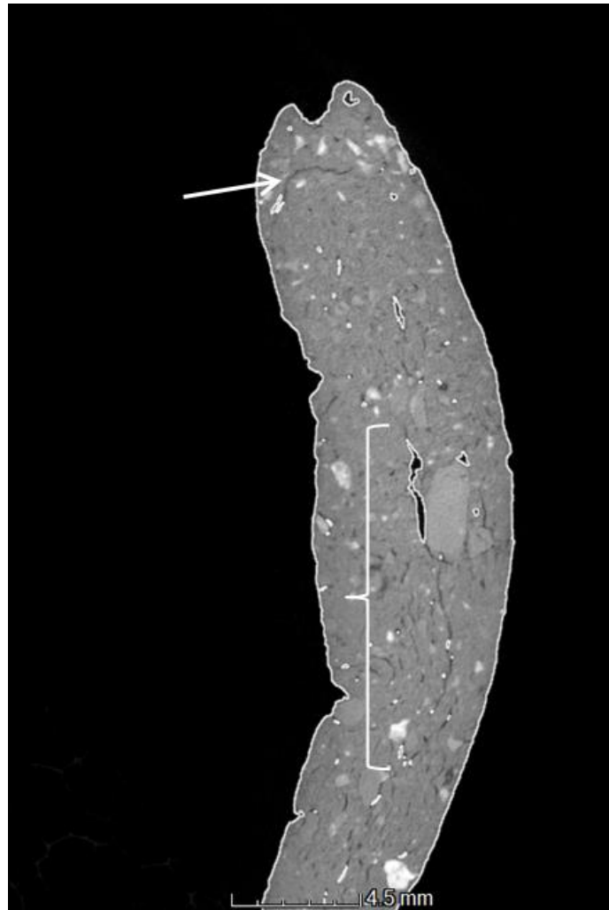
Figure 6.30: Specimen 043. No castellation is present, but there is clay added consistently along the lip of the vessel above a fold. The large vertical void indicated by the bracket is from clay layers not being fully compressed while folding, and the horizontal void indicated by the arrow is the joining where the extra clay was added to the lip of the vessel.
