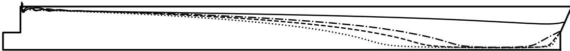
Figure 4.15: Representative 3D stagnation streamlines of the k-\epsilon (dotted), k-\omega (dashed), k-\omega SST (dash-dotted), and SAS SST (solid) simulations which have been 'unwound' from the tube axis. The tube aspect ratio ( L/D ) has been decreased by a factor of 4 to emphasize the differences in streamline position.
