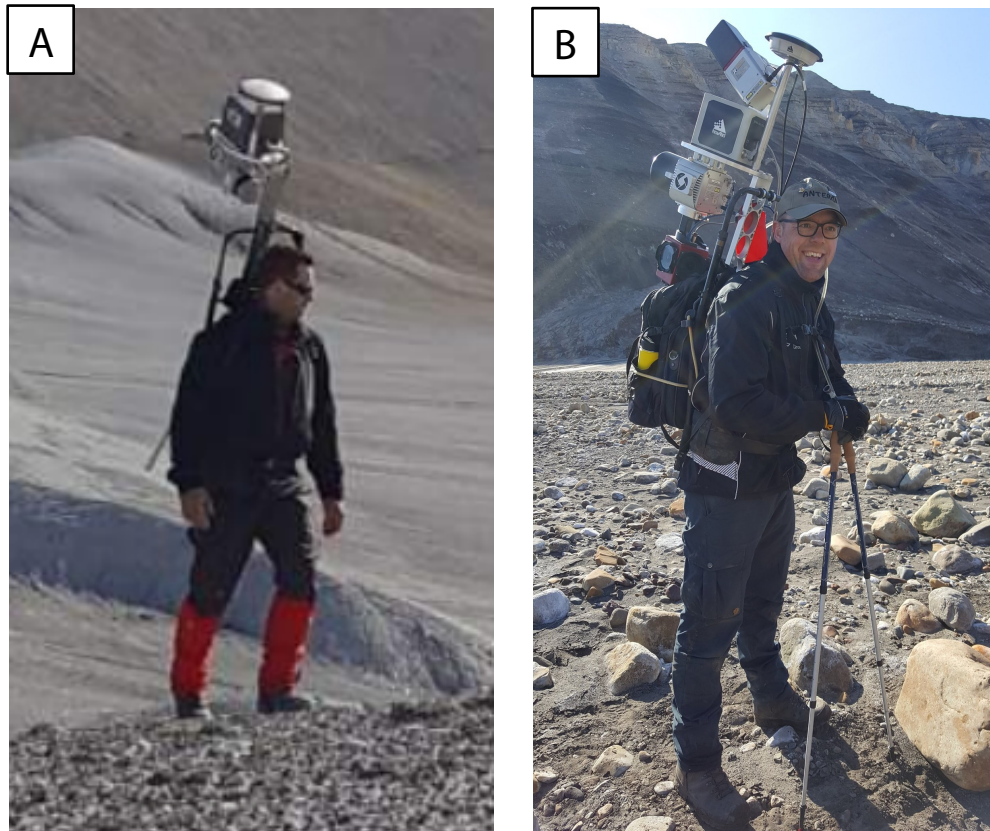
Figure 1.7. (A) 2016 field team member (Michael Zanetti) traversing with the Akhka-R3 Kinematic Lidar System (KLS) in the Houghton Impact Structure on Devon Island in the Canadian High-Arctic (B) Prof. Antero Kukko traversing with the AkhkaR4DW Backpack mobile laser scanning system in the Mokka Fiord Valley on Axel Heiberg Island in the Canadian High-Arctic in 2018.
