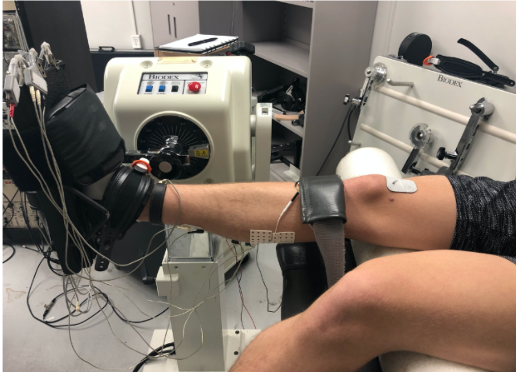
Figure 3. Experimental setup for fatigue protocol. Participant's right foot secured against footplate with right ankle slightly dorsiflexed, knee and hip fully extended.
