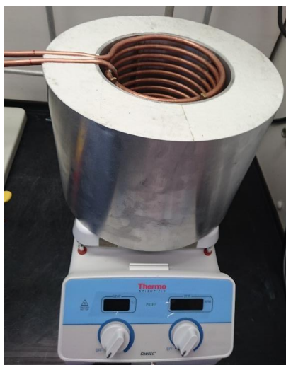
Figure 73. Water-cooled heat exchanger in CREC-VL-cell
