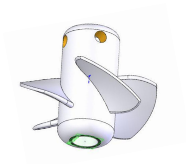
Figure 23. Description of Marine Type Impeller Used in the CREC-VL-Cell
