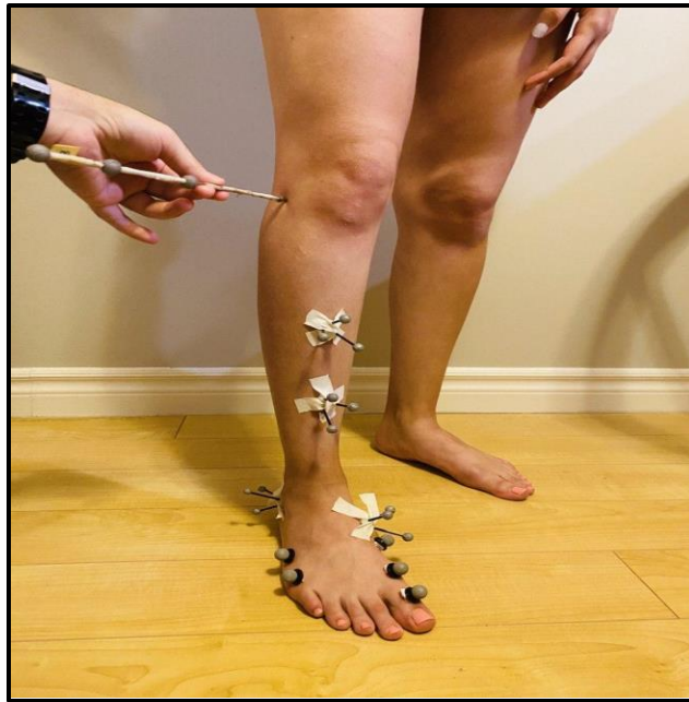
Fig. 2-4: Digitizing landmarks. Holding a wand against the position of a bony landmark for digitizing a landmark.
