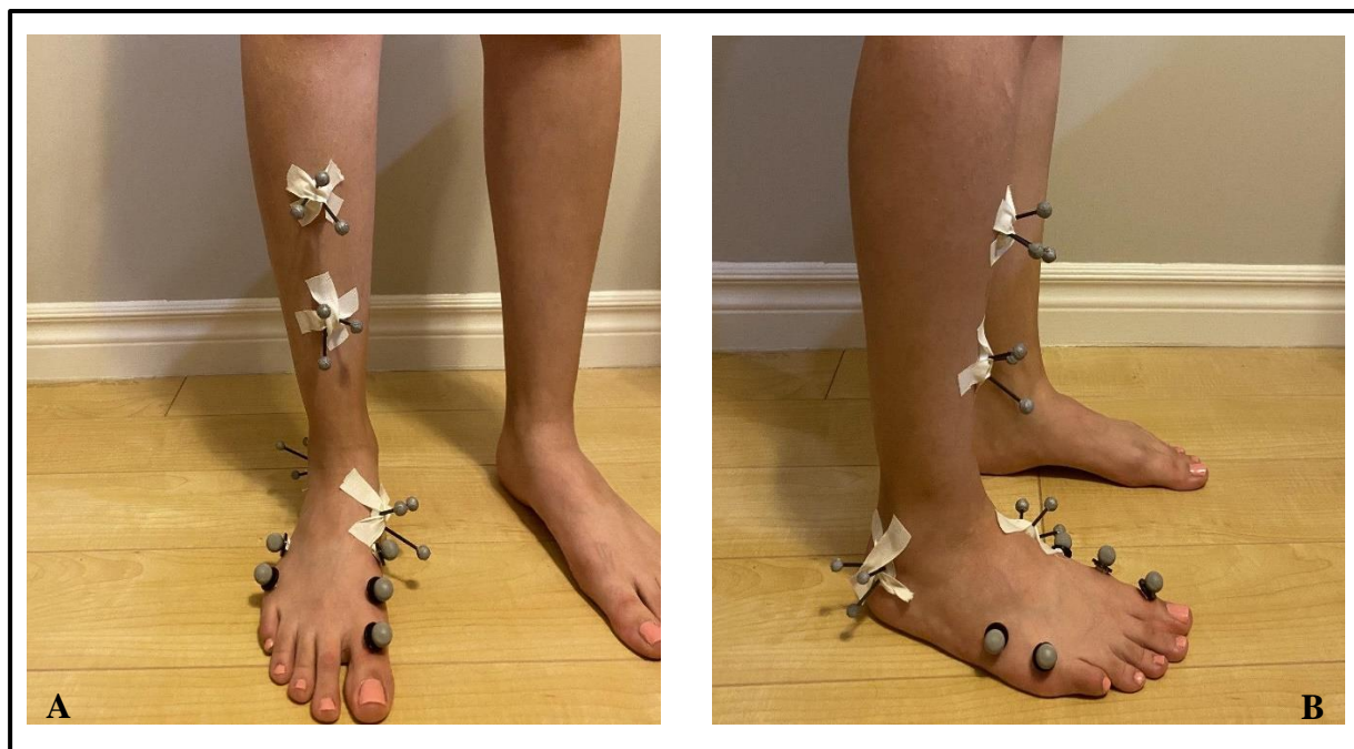
Fig. 2-2: Jenkyn and Nicole's model marker set. A) Frontal view and B) lateral view of the MSFM marker-set configuration used for this study.
