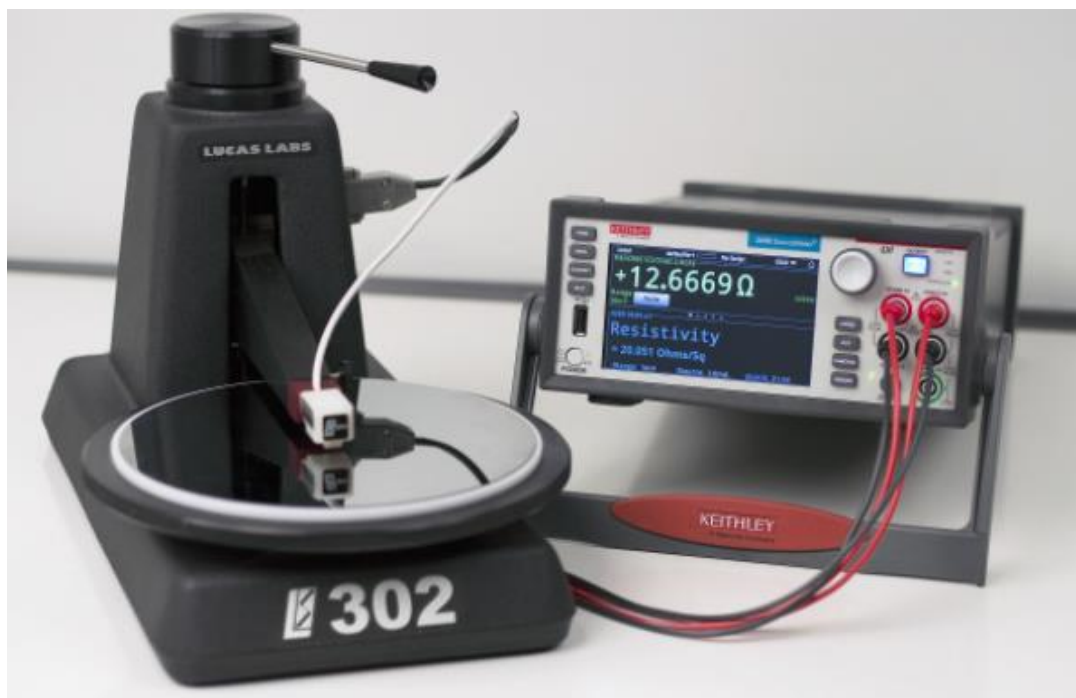
Figure 47 Model 2450 SourceMeter SMU Instrument with the Lucas/Sigmatone Corporation (Gilroy, CA), Model SP4 4-Point Probe Head and S-302 Test Stand measuring the conductivity of a sample.
