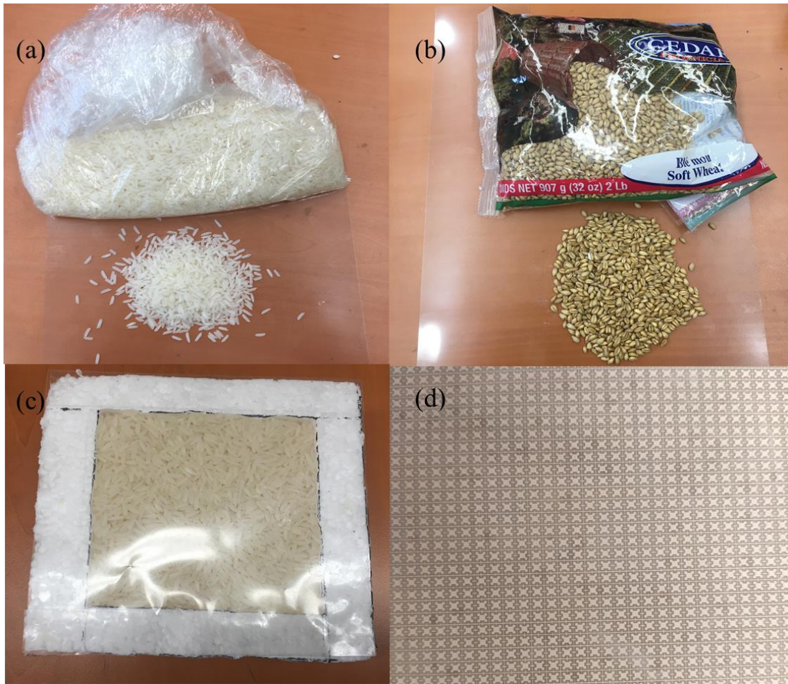
Figure 72 Materials used in the test: (a) rice; (b) soft wheat; (c) food container; (d) metasurface.
