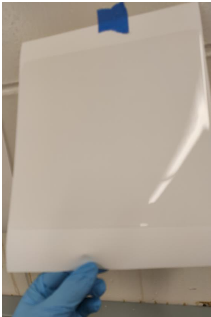
Figure 35 Wet film of the Vc coating with the mirror-like surface.
