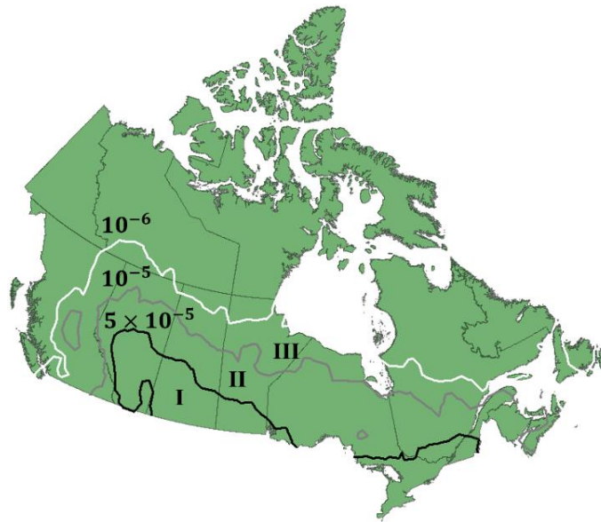
Figure 4.7. Identified contour lines with the annual mean tornado occurrence rate (per \text{km}^2 per year) equal to 5 \times 10^{-5} , (I: Region prone to significant tornadoes), 10^{-5} (II: Region prone to tornadoes), and 10^{-6} (III: Region with rare tornado occurrence).
