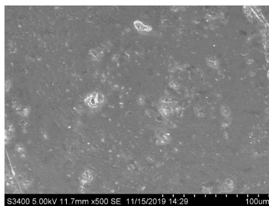
Figure S7.9 The SEM images of cycled Na@alucone electrode that obtained from Na-O 2 battery using SSE.
