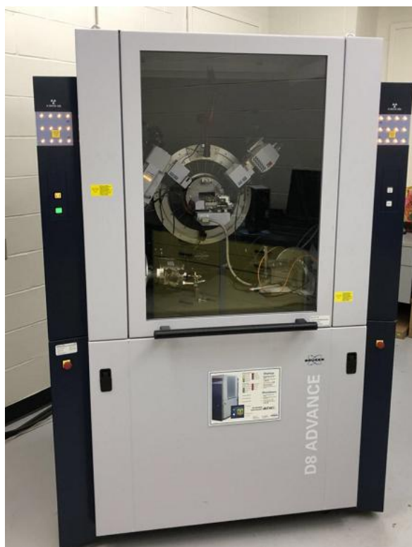
Figure 3.5 The Bruker D8 Advance XRD with Cu- K\alpha radiation.
