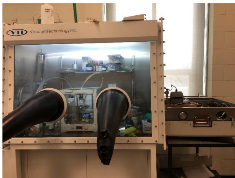
Figure 3.3 The Gemstar-8 ALD/MLD system connected with Ar-filled glove box (Arradiance, USA).
