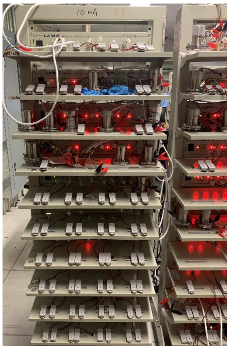
Figure 3.7 Photo image of a group of Land 2001A Battery Test Systems. Each unit has 8 independent channels for battery testing.
