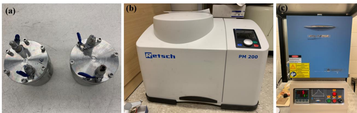
Figure 3.2 (a) A pair of zirconia vessels (out-shell with stainless steel), (b) Ball mill machine for rotating the zirconia vessels. (c) High temperature Muffle furnace for SSE sintering.
