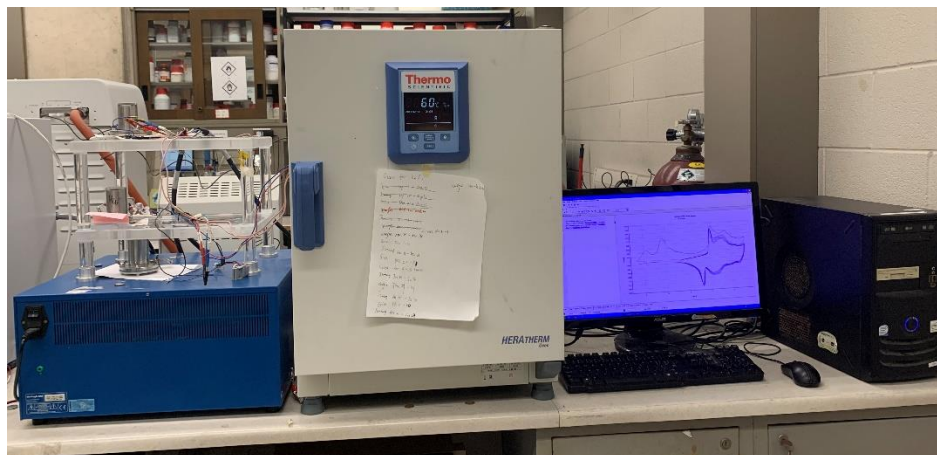
Figure 3.8 Photo image of A multichannel potentiostat 3/Z (VMP3) coupling with an oven for temperature variation testing.
