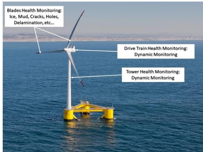
**Figure 2.11: Sensors for WTHM.**
