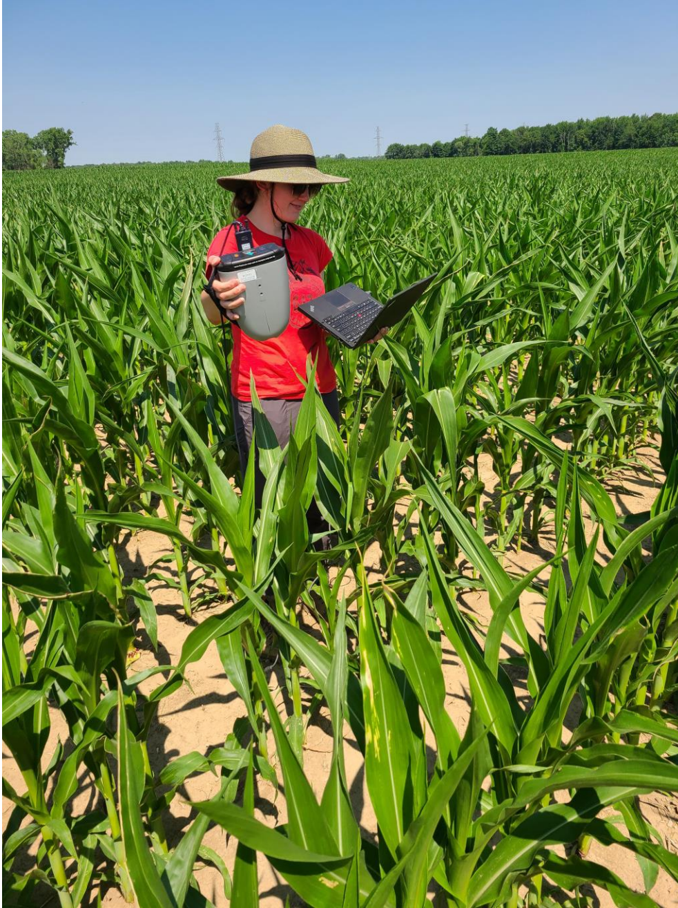
Figure B-6. Retrieving spectral reflectance data from corn using ASD (Robin Kwik, GITA lab)
