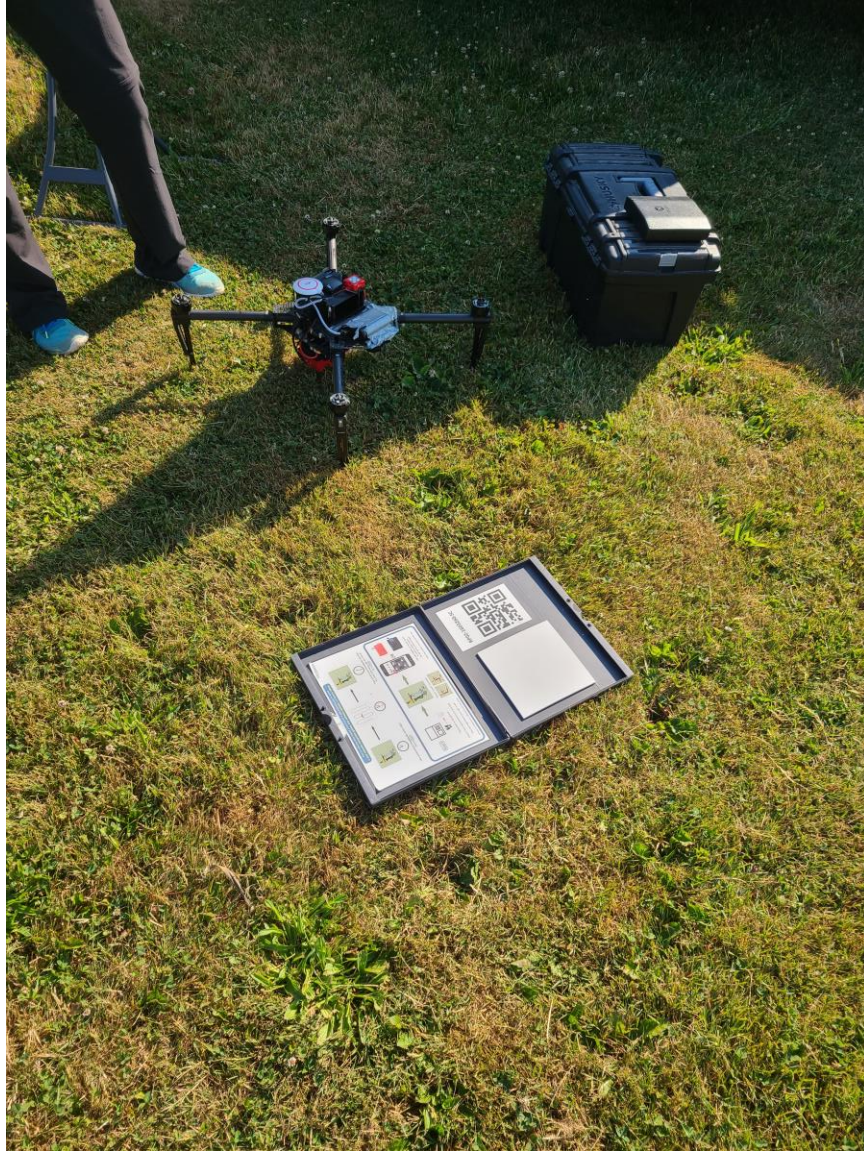
Figure B-7. UAV (DJI Matrice 100) prior to take-off. Calibration panel is shown beside
