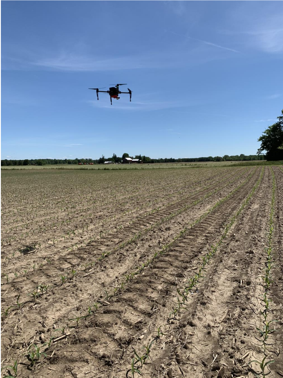
Figure B-8. UAV (DJI Matrice 100) flying over corn field at early growth stage
