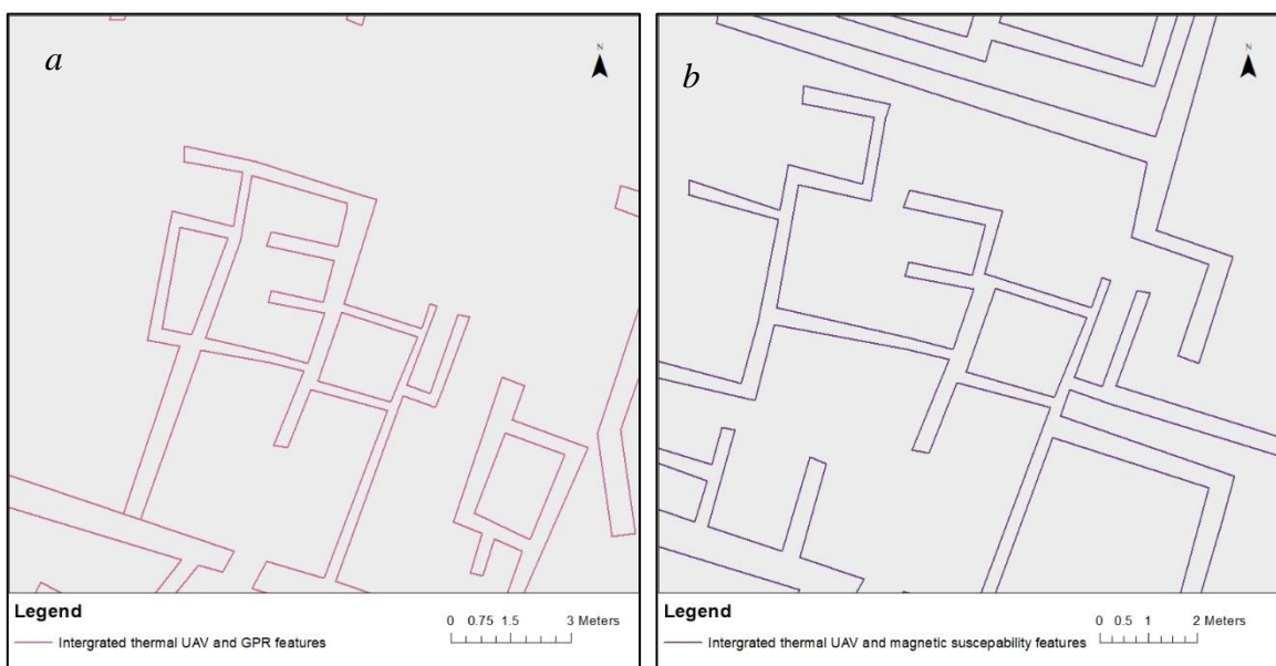
Figure 5.8: (a) Comparison of thermal with GPR results; (b) thermal with magnetic susceptibility results.
