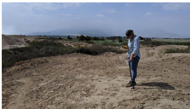
Figure 4.3: Barrington MS3 susceptibility meter with an MS2D surface scanning probe. Photo by Edward Eastaugh.
