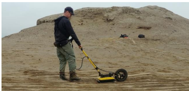
Figure 4.25: Noggin 500® with a SmartTow configuration. Photo of Edward Eastaugh by Kayla Golay Lausanne.
