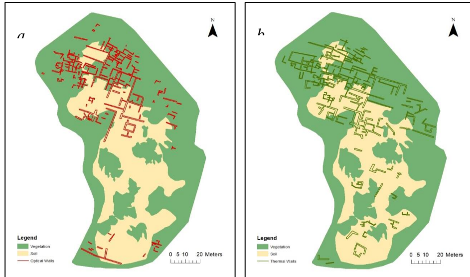
Figure 5.3: Aerial survey comparison, vegetation versus soil. (a) Optical UAV survey; (b) Thermal UAV survey
