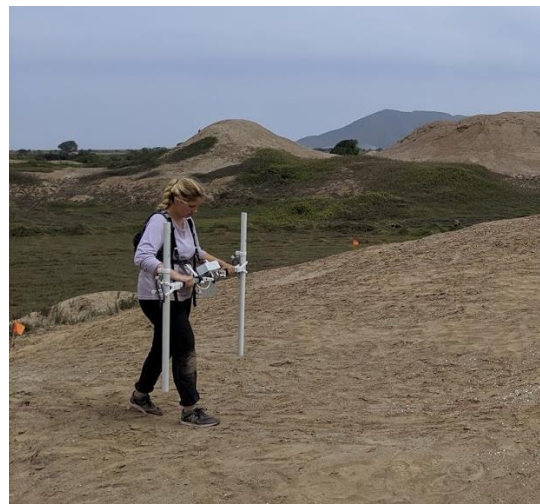
Figure 4.14: Bartington Grad601-2 dual-sensor Fluxgate Gradiometer. Photo by Edward Eastaugh.
