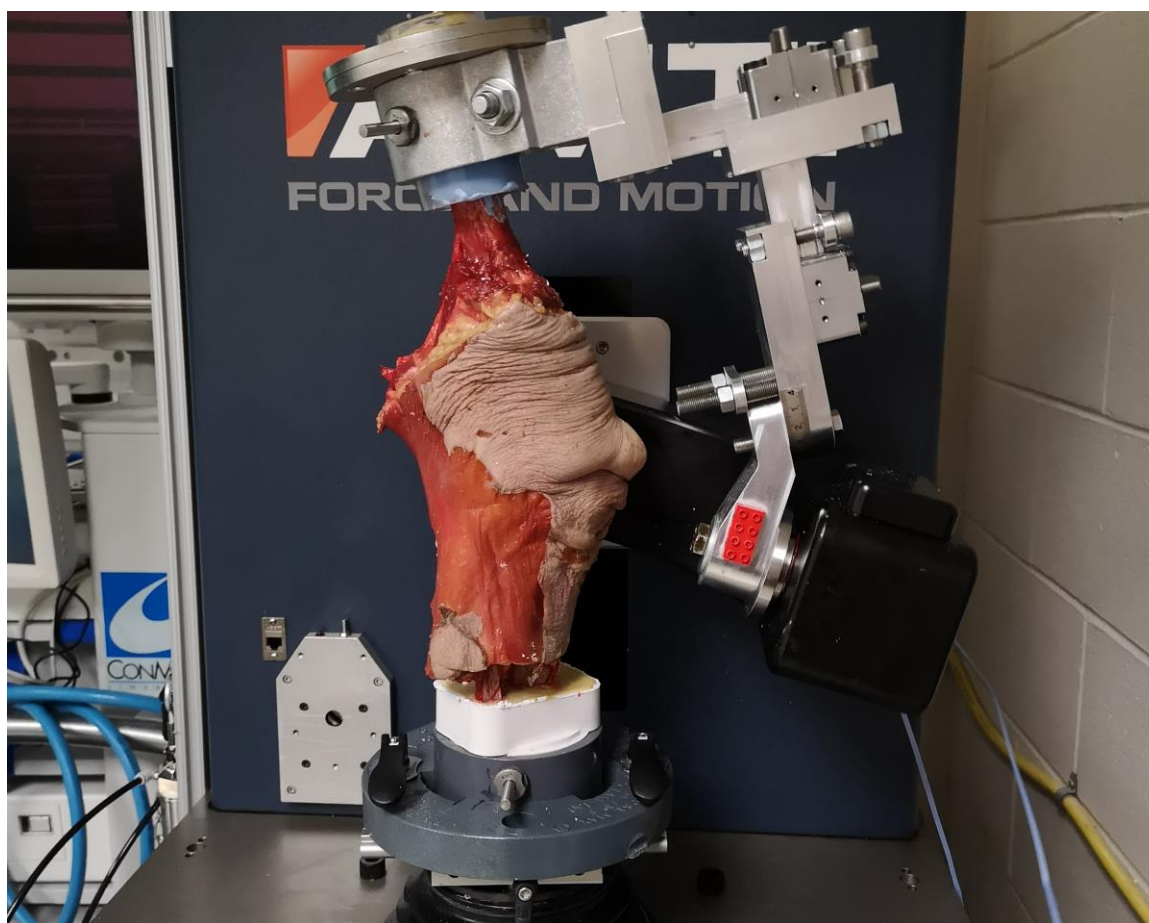
Figure 3.5—Depiction of the cadaveric knee with the installed articulating spacer and sensors mounted to the VIVO apparatus for the purposes of anatomic loading.
