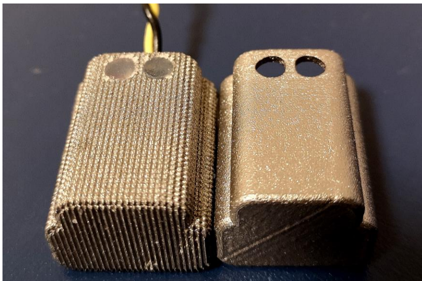
Figure 2.5—Two titanium superstructures, pictured with the intentionally textured pattern (left) and the smooth alternative (right).
