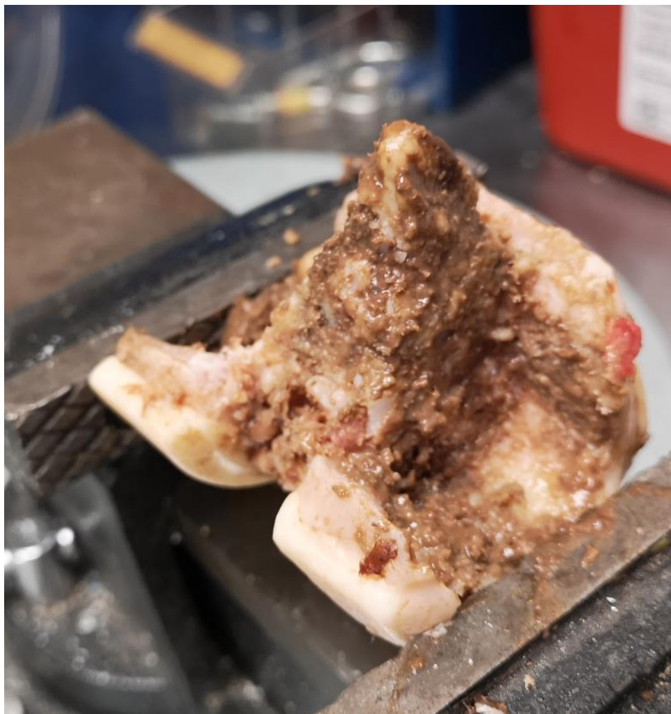
Figure 3.18—Explanted femoral spacer component clamped in a bench vice displaying superior bone cement coverage of the sensing package.
