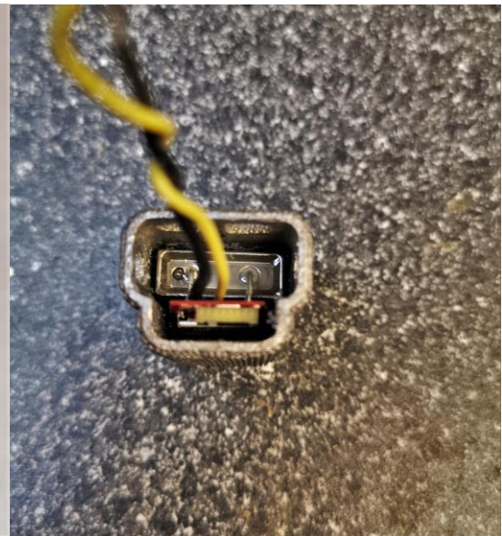
Figure 2.8—The fixture is removed following Step 5 with the package suspended by cured first stage.
