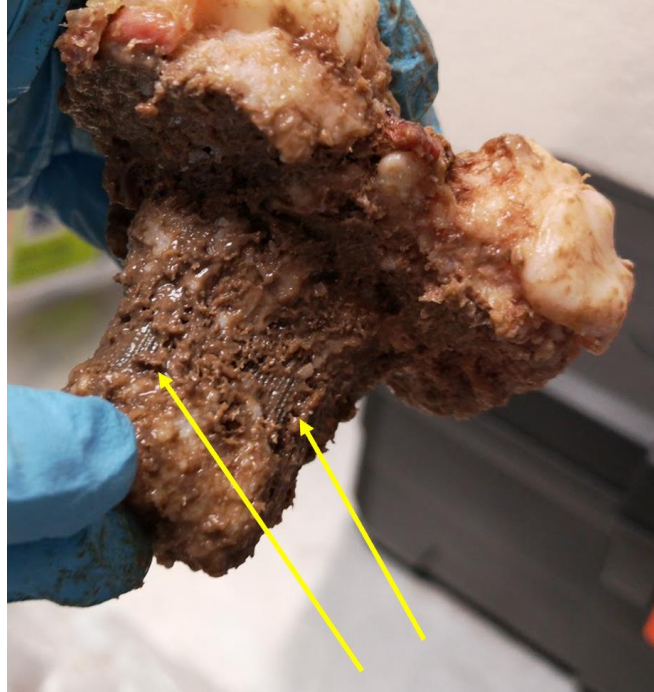
Figure 3.16—Two areas with insufficient bone cement can be observed on the tibial keel.
