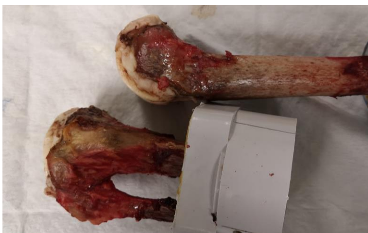
Figure 3.13—An auxiliary view of the tibia and femur following the loading cycles and debridement. No spacer separation or major fracturing was observed.
