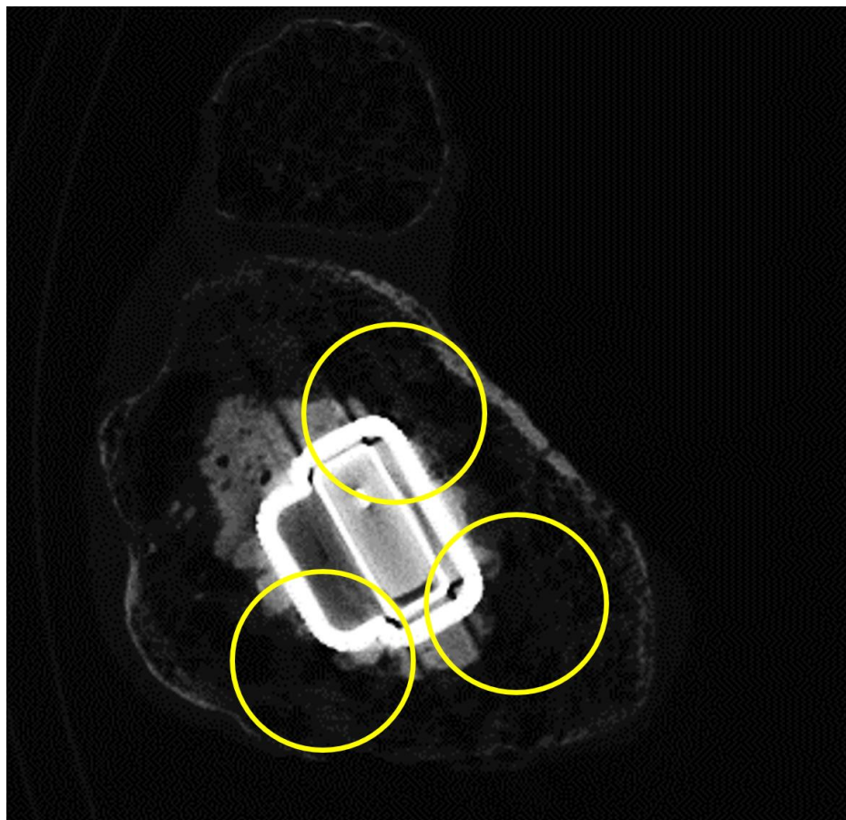
Figure 3.15—Micro CT image depicting a sagittal view of the tibial implant where three regions of poor bone cement integration with the implanted instrumentation can be observed.
