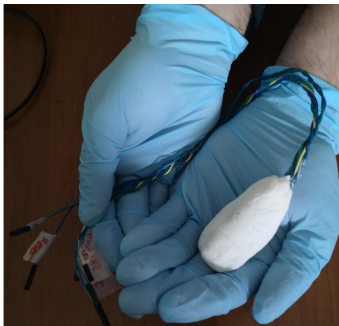
Figure 3.1—Specimen B, an encapsulated sensing package, which has been potted in bone cement to demonstrate similar thermal insulation characteristics to the implanted embodiment.
