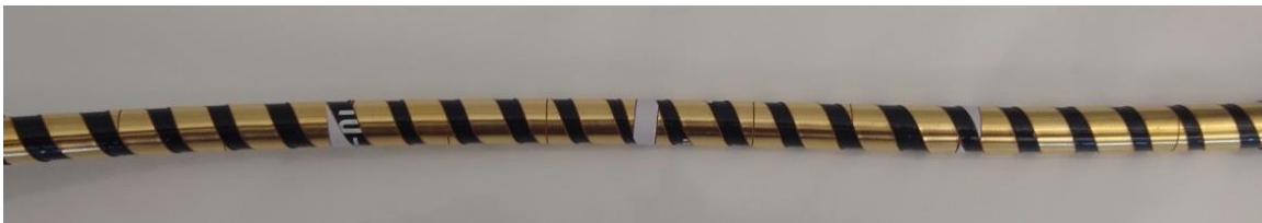
Figure 3.2 - Helical sensorized sleeve design
