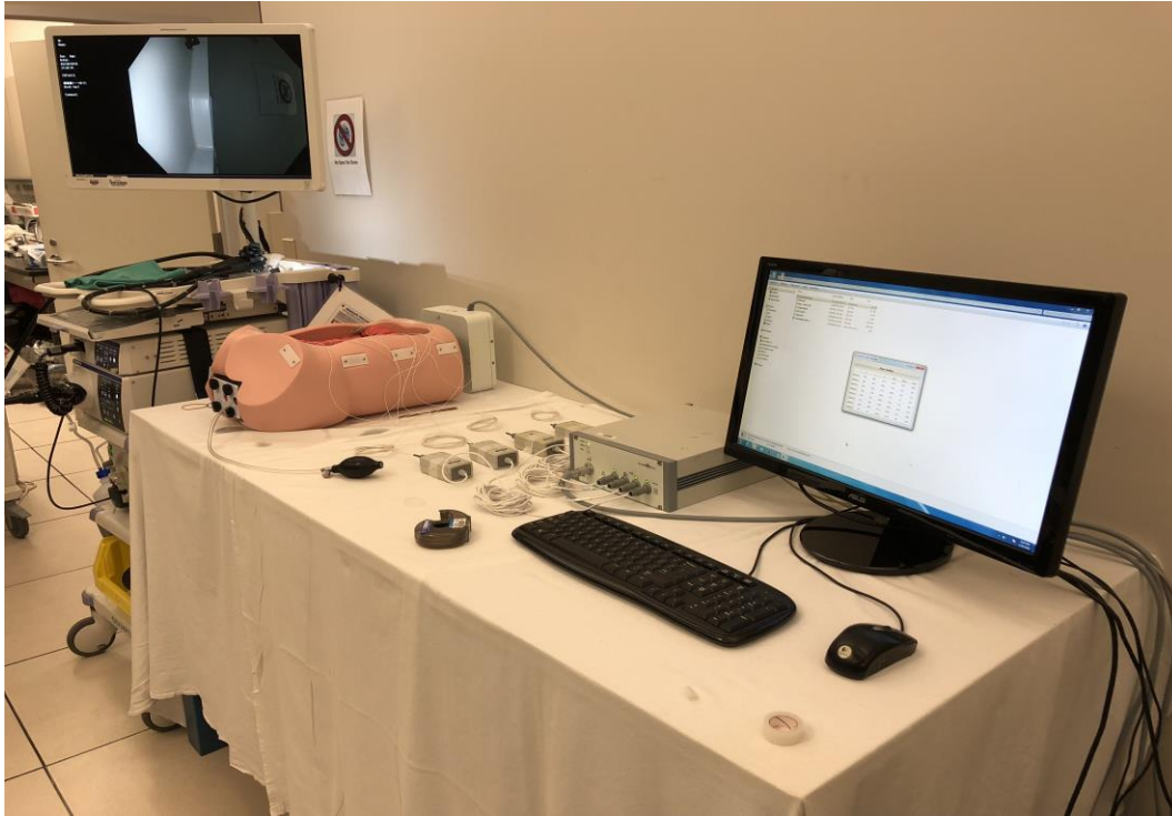
Figure 2.1 - Experimental setup for the colonoscopy simulation model
