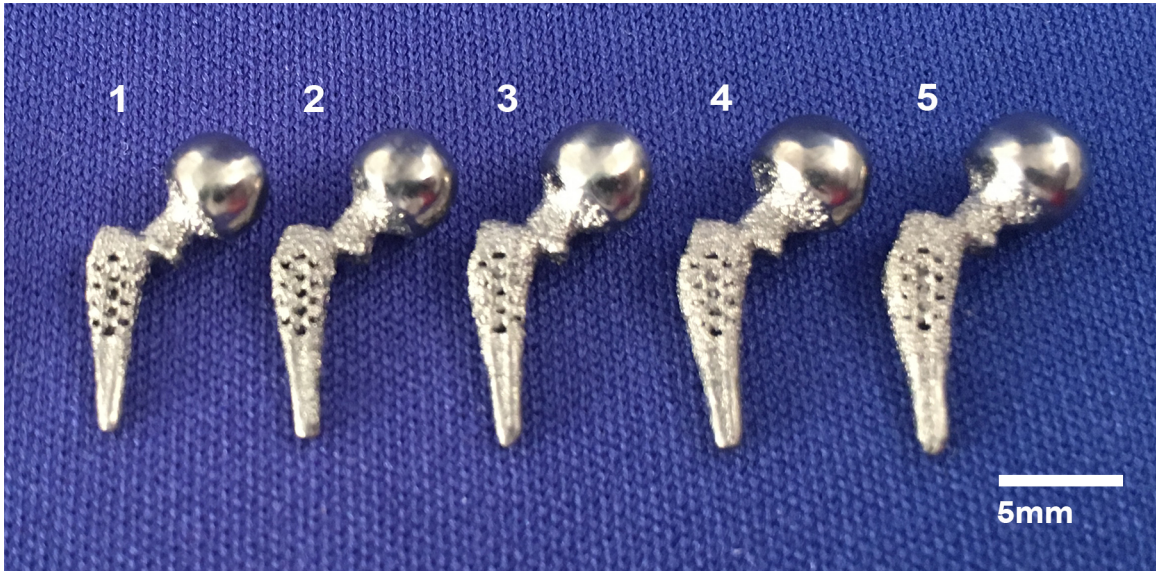
Figure 2.8: Generation 2 rat-specific 3D-printed implants. Five sizes (1-5) were created to accommodate a range of skeletally mature rats (male, Sprague-Dawley, 390-605g). Implants shown were 3D-printed in Ti6Al4V titanium with heads polished to a mirror-like finish with a dental tool and progressively finer grits of polishing stones and rubber wheels.
