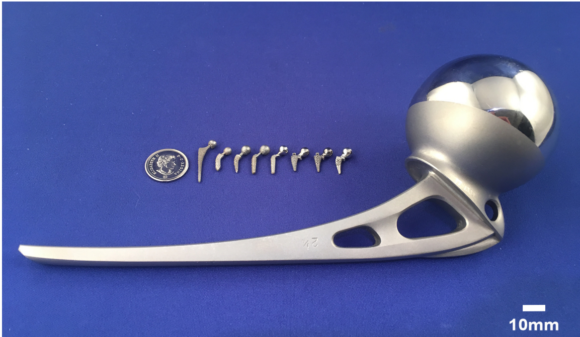
Figure 5.4: An Austin Moore unipolar femoral hip hemiarthroplasty prosthesis beside an array of unipolar rat hip hemiarthroplasty implants in various medical grade alloys, and a Canadian dime for scale. Numerous implant iterations were created and tested before arrival on our final implant design.
