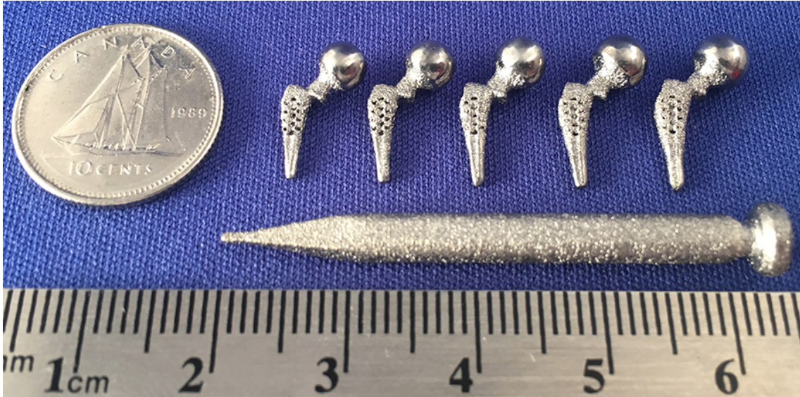
Figure 3.1: Custom rat hip implants created in medical-grade titanium alloy (Ti6Al4V) in a range of sizes to accommodate rats of various weights, shown beside a Canadian dime for scale. A hexagonal porosity was introduced into the stem design (0.5mm diameter) in an effort to facilitate osseointegration. A collar was included to help prevent over-pressing of components and aid in primary stability. An impactor tool was also printed to facilitate the press-fit of implants into the medullary cavity.
