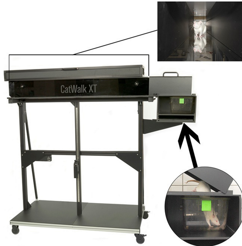
Figure 1.4: CatWalk XT system (Noldus, Leesburg, Virginia) for murine gait analysis. The system includes a glass-floored walkway, with one open end; the other end contains an enclosure that houses the animal's cage. A camera captures fluorescent light that is reflected downward when the animal makes contact with the glass floor. Image is reused from Kappos et al 2017; 84 an open-source article published by John Wiley and Sons and distributed under the terms of the Creative Commons License, CC BY (see: creativecommons.org/licenses/ ) (copyright license not required to reuse in this thesis).
