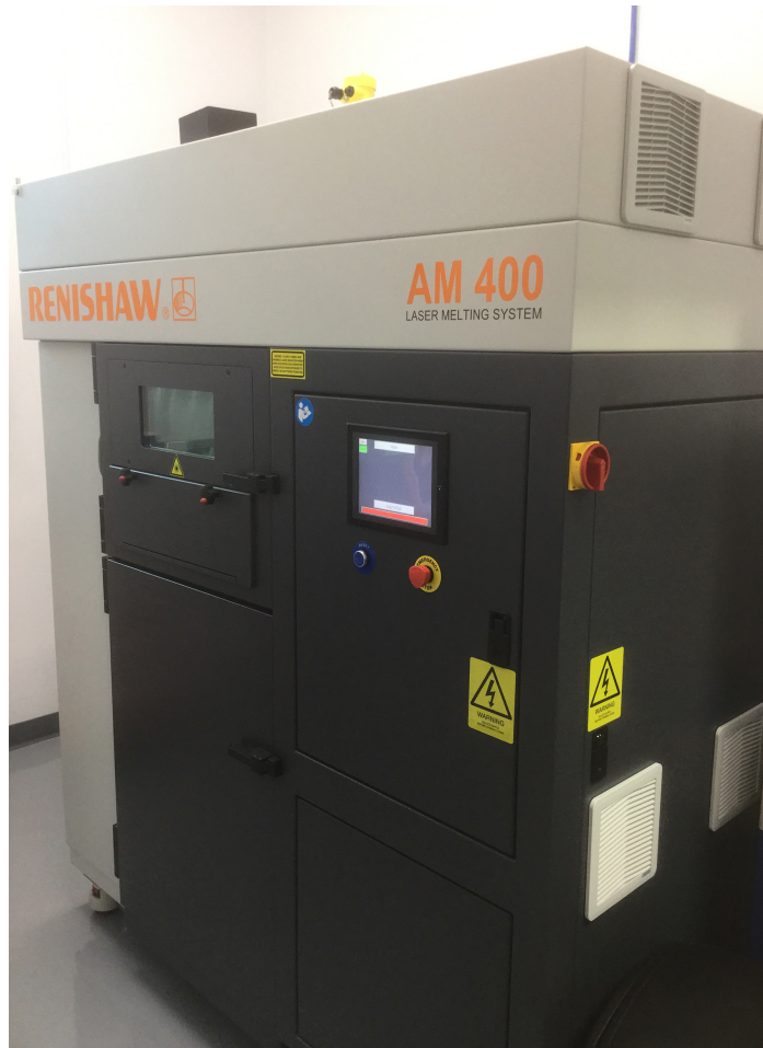
Figure 1.2: A Renishaw plc AM 400 selective laser melting 3D printer (ADEISS Canada, London, Ontario) capable of building parts in medical-grade metal alloys.
