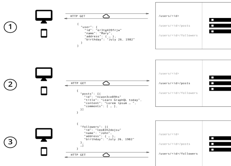
Figure 4.5: With REST, 3 requests are made to fetch data from 3 different endpoints. Also, it over fetches data with additional information. Image Adapted from [90].
