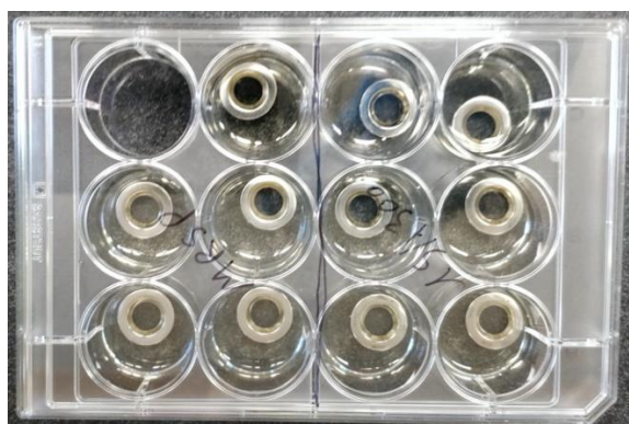
Figure 2 - Sterilized washers placed into the wells of a 12 well tissue culture plate.
