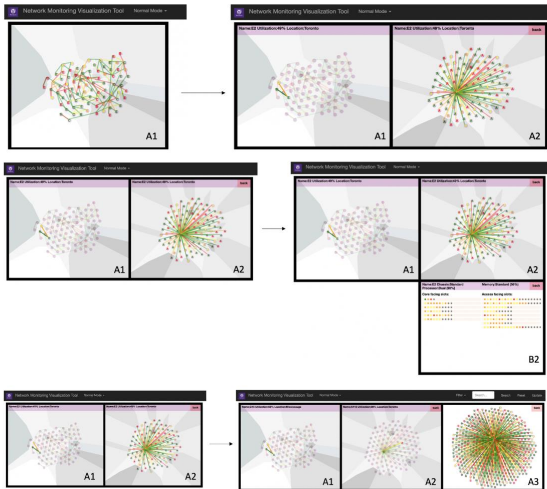
Figure 22: a- Clicking the edge router in the A1 panel (Up); b- Clicking the edge router in the A2 panel (Middle); c- Clicking the access router in the A2 panel (Down)
