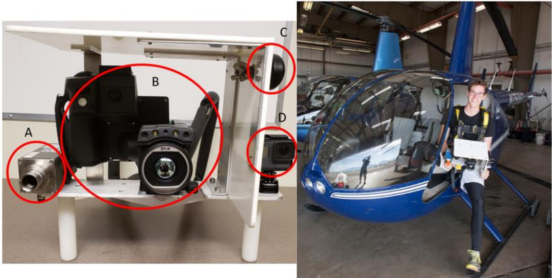
Figure 2.6 Photos of (a) the instruments affixed to the operator mount: A is the Heitronics KT15.82 infrared radiometer, B is the FLIR T650 thermal imager, C is the Aaronia GPS Logger, and D is the Go PRO Hero 5 and (b) the operator mount as utilized from the helicopter.
