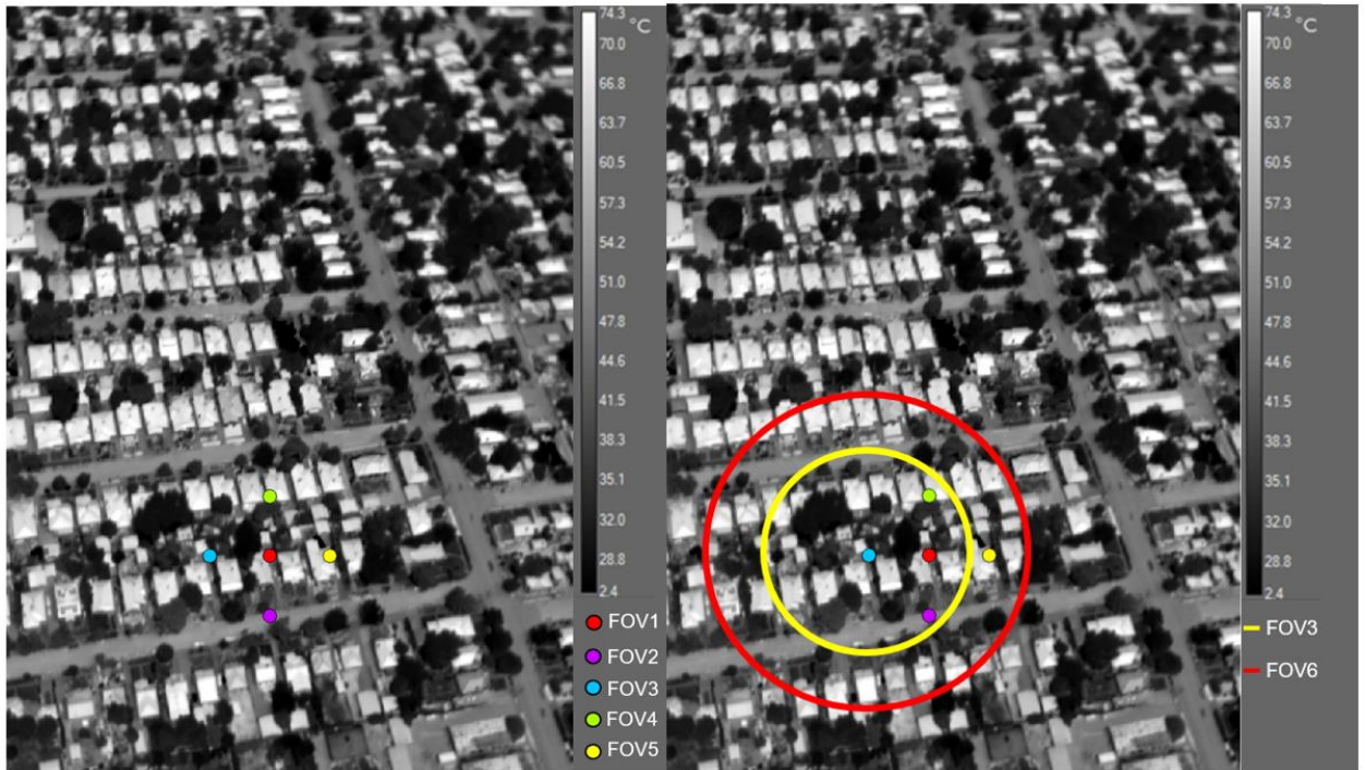
Figure A.5 Sample thermal image from LW12 showing (left) the center points of FOV1 – 5 with FOV1 being the lab determined IFOV_{KT15.82} and (right) FOV6 and FOV7 showing the increase and reduction of FOV3 (the location of best match).
