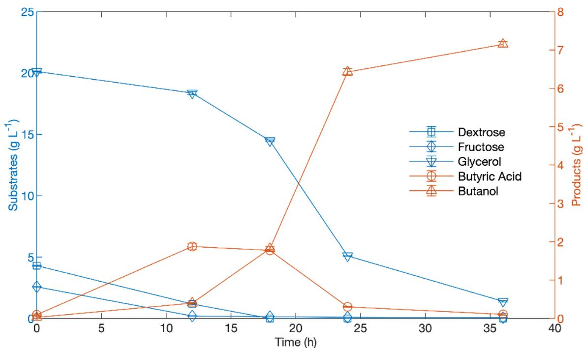
**Figure 2.5:** Fermentation products at the optimum glycerol:molasses ratio. Butyric acid is produced from the sugars present, then subsequently taken back up by the cells to increase the productivity of butanol. Conditions were tested in triplicate with the mean of the results presented. Error bars represent standard deviation from the mean.
