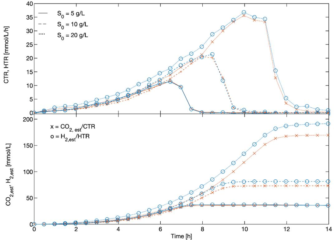
**Figure 4.3:** Top: CTR and HTR profiles of fermentation with *C. pasteurianum* in medium containing 5, 10, and 20 g/L glycerol as the carbon source.
