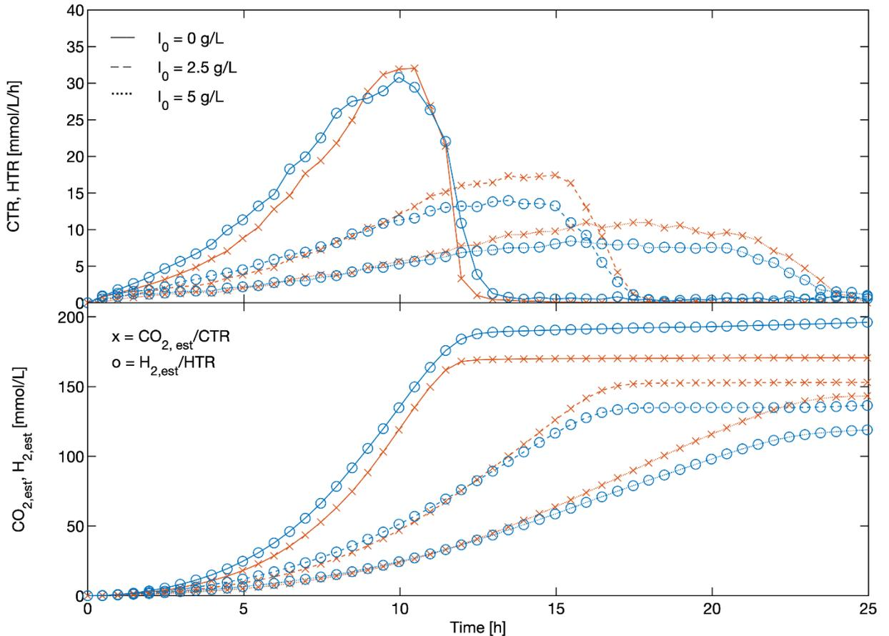
**Figure 4.4:** Top: CTR and HTR of inhibited *C. pasteurianum* fermentation due to increasing concentrations of butanol added ( $I_0$ ) to medium at time of inoculation.
