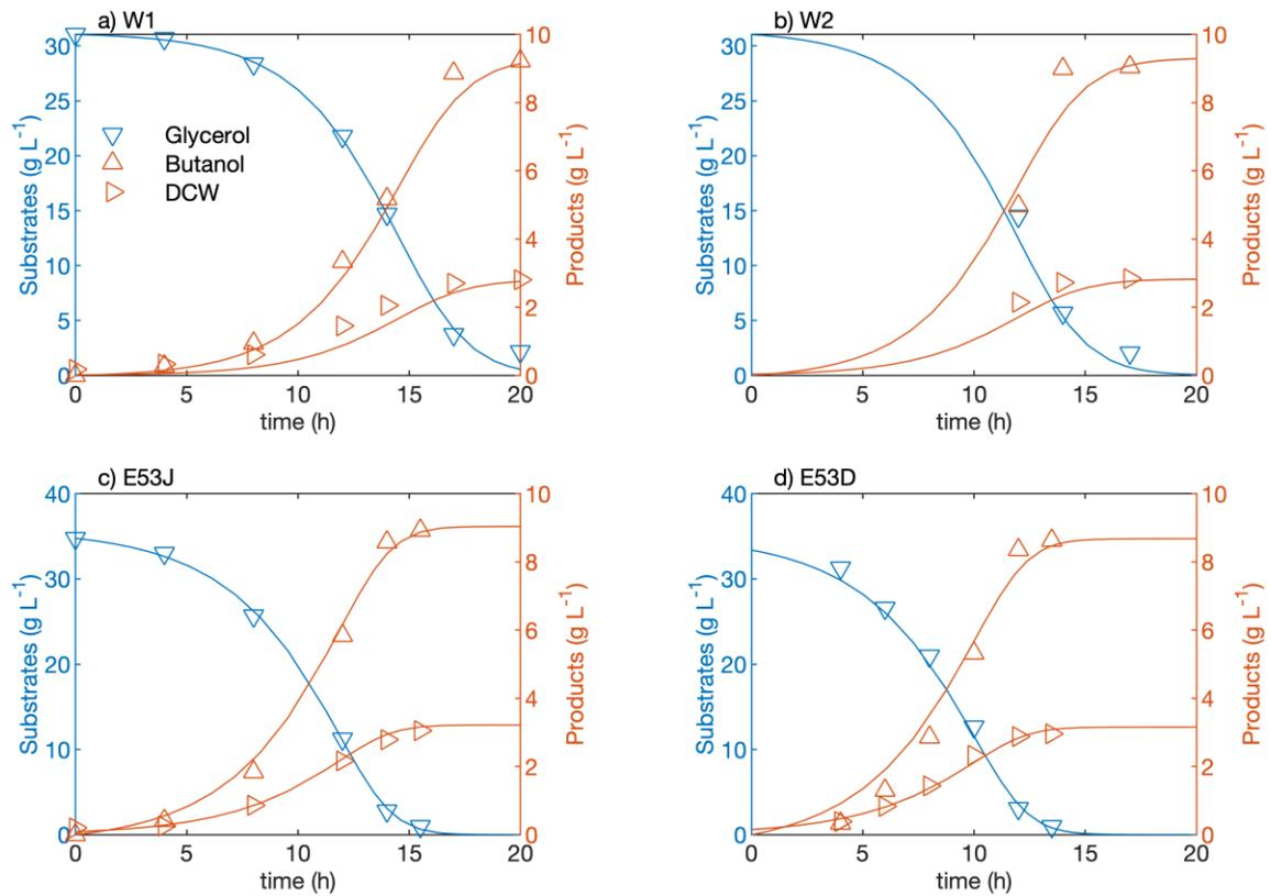
**Figure 3.1:** Glycerol consumption, butanol and cell biomass production over time of reactor-scale fermentations using two *C. pasteurianum* wild-type samples (top, graphs A and B) and two putative mutant samples (bottom, C and D). Solid lines are the best fit results for the consumption of glycerol and production of butanol and cell biomass.
