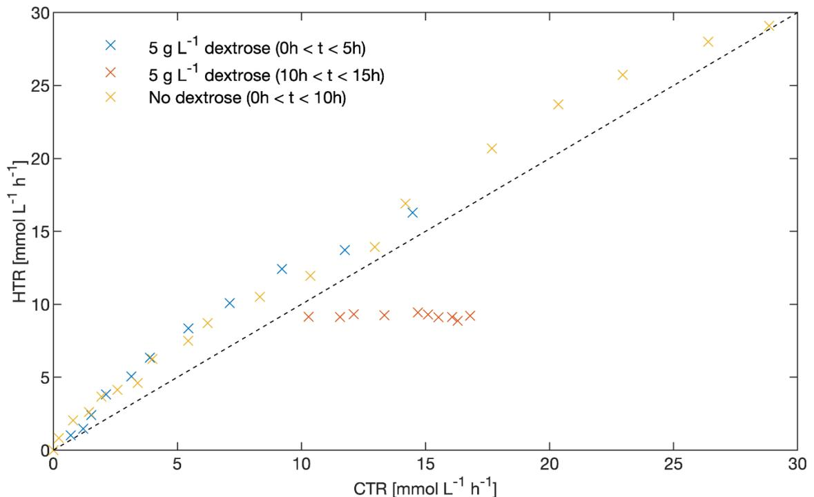
**Figure 4.6:** CTR vs. HTR of *C. pasteurianum* fermentations containing only glycerol as the carbon source (dark squares) or a mix of glycerol and dextrose. The 0 g/L dextrose sample shows the ratio of CTR/HTR remaining consistent through the course of the fermentation. The 5 g/L dextrose initially follows a similar trend (0 to 5 hours), however following the depletion of dextrose in the medium (10 to 15 hours) the CTR/HTR trend differs greatly.
