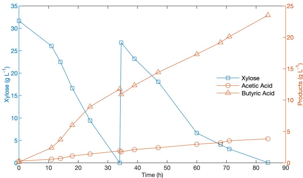
**Figure 2.1:** Xylose consumption and product formation in a fed-batch fermentation strategy of *C. tyrobutyricum* to produce butyric acid rich supernatant. Culture was grown in a 7L reactor with a 5L initial filling volume, and maintained at a pH of 6.3 to select for butyric acid production. Final values for detectable products were (in g/L): butyric acid = 23.5; acetic acid = 3.8.
