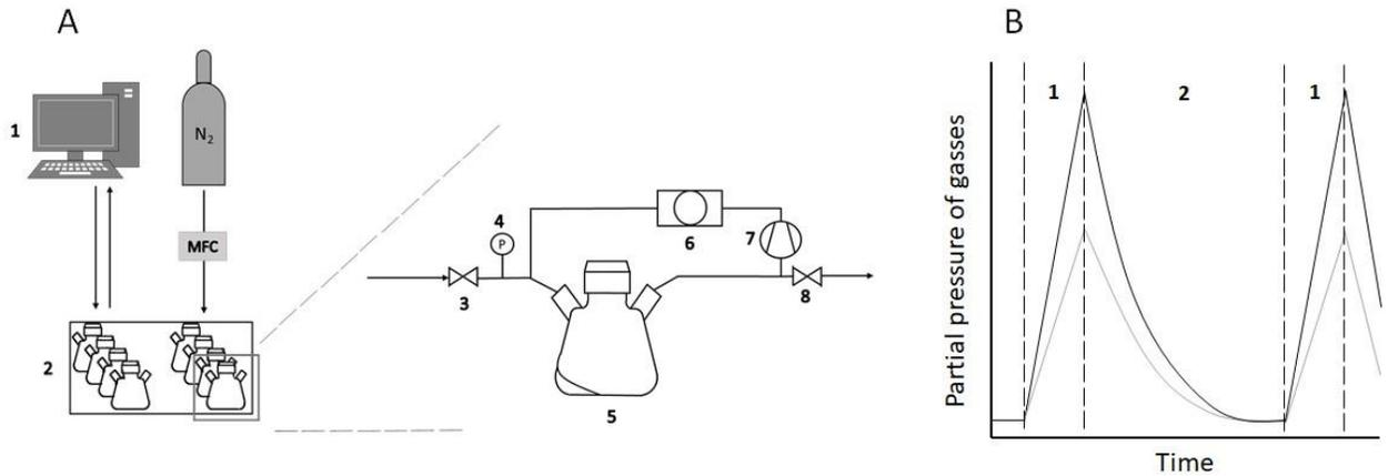
**Figure 4.1:** A) Schematic overview of the anaRAMOS system and details on single flask/sensor arrangement. 1: Computer controlling valves and logging CTR data. 2: Heating/shaking unit containing 8 anaerobic flasks in a parallel system with RAMOS circuitry board installed. 3: Gas inlet control valve. 4: Pressure sensor 5: anaRAMOS flask with culture. 6: CO<sub>2</sub> sensor connected to central circuitry. 7: Micropump. 8: Gas outlet control valve.
