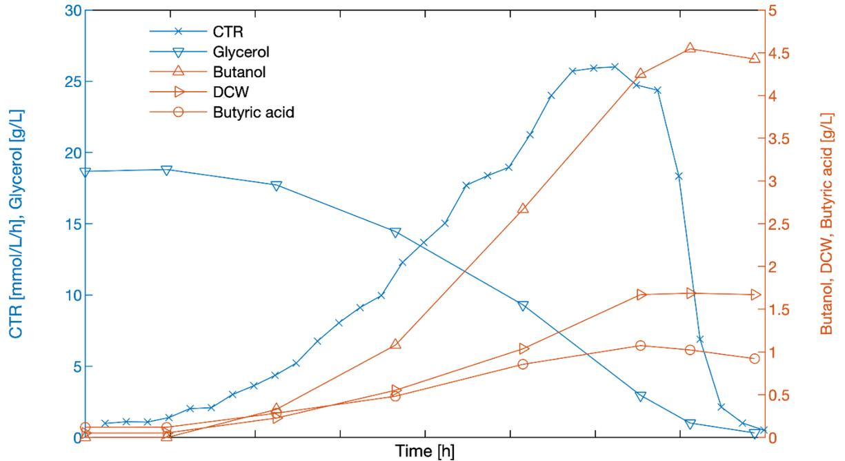
**Figure 4.2:** Example data from single run of the anaRAMOS demonstrating combination of online and offline signals obtained at the shake flask scale. Fermentation volume was 30 mL, which initially contained 20 g/L glycerol and was incubated at 35°C at 100 RPM.
