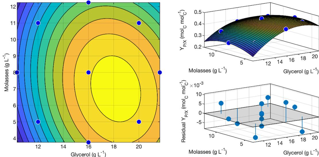
**Figure 2.4:** Surface and residual plots of effects of amount of glycerol and molasses in starting medium on the relative carbon yield.
