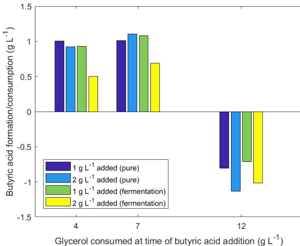
**Figure 2.3:** Comparison of the amount of butyric acid produced or consumed when added during fermentation with differing amounts of remaining glycerol.
