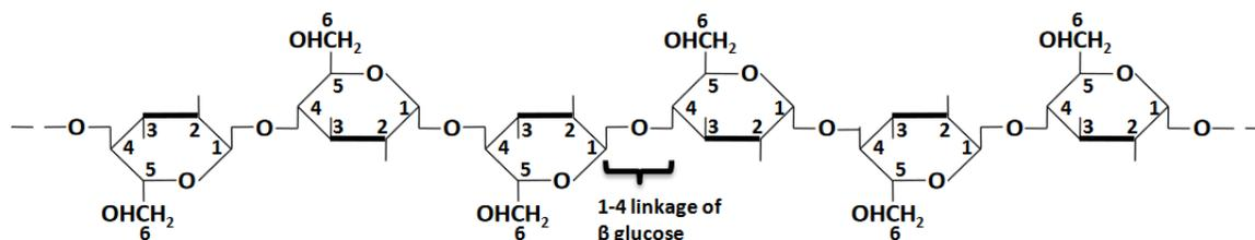
**Figure 1.1:** Molecular structure of cellulose (adapted from O’Sullivan 1997)
