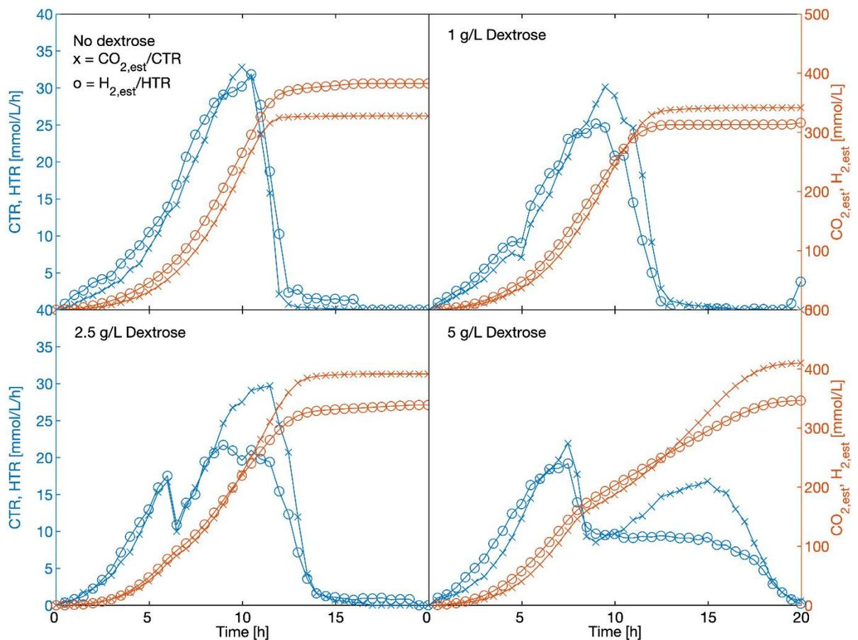
**Figure 4.5:** CTR, HTR, CO<sub>2</sub> production, and H<sub>2</sub> production over the course of *C. pasteurianum* fermentations containing 20 g/L glycerol and varying amounts of dextrose in the starting medium. Sharp decrease in CTR and HTR indicate time of dextrose depletion in medium. Lines marked with an x are the CTR and CO<sub>2</sub>, lines marked with open circles are
