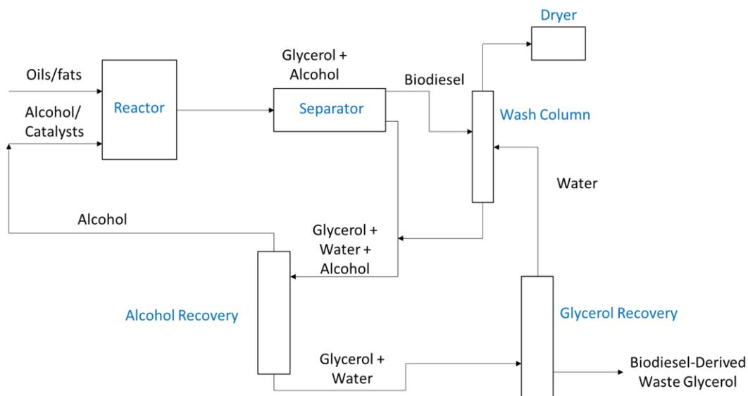
**Figure 1.2:** Flow diagram overview of a standard conversion of oil and fats to biodiesel
