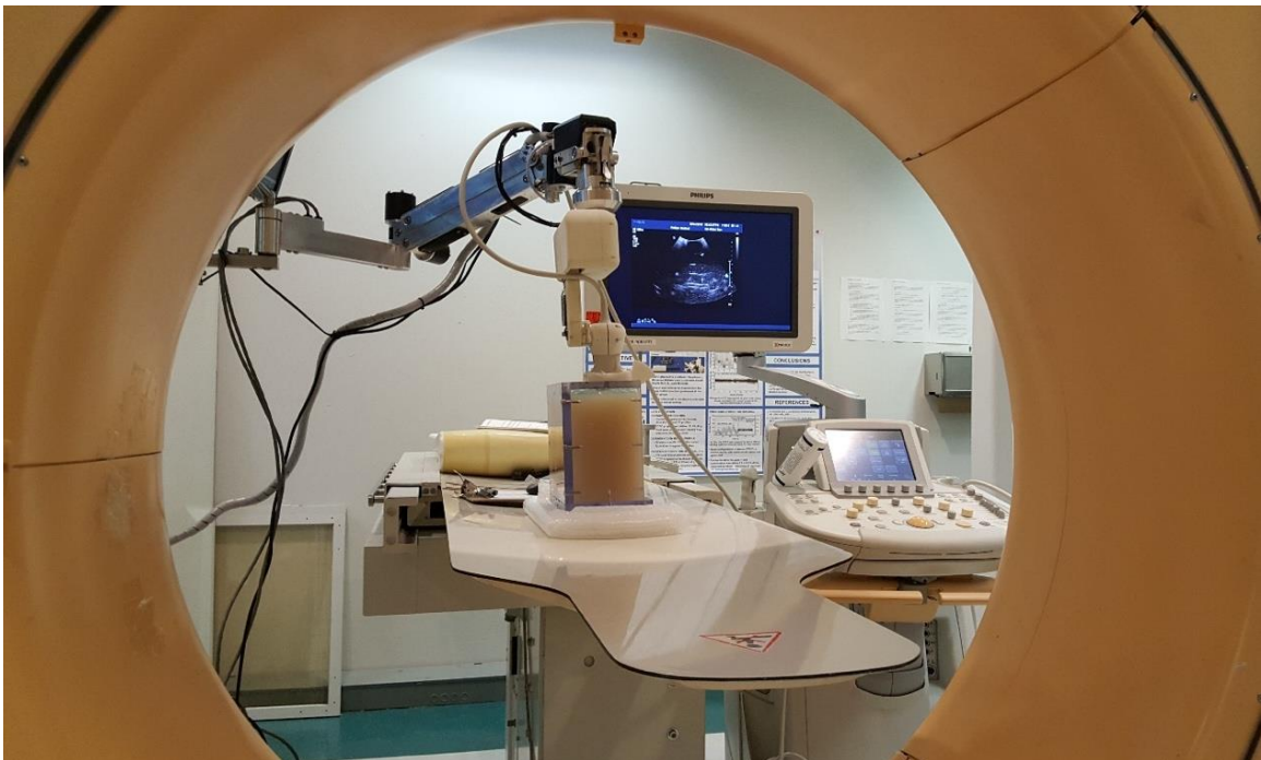
Figure 4.4 Experimental set-up for a 3D US image-guided needle insertion with an O-arm providing external imaging comparison for targeted needle placements.
