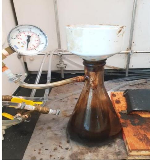
Fig. 3.1. Vacuum filter assembly for the asphaltenes concentration measurement
