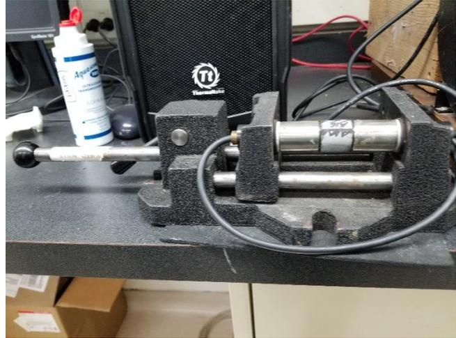
**Figure 2.5: Photos of laboratory rock sample  $V_p$  measurements showing a) the whole apparatus and b) a clamped 1-cm cylindrical sample from station A16.**
