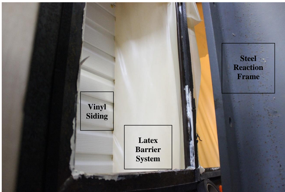
Figure 2.12: A photograph showing the latex barrier system, creating separate airboxes attached to a vinyl siding specimen.
