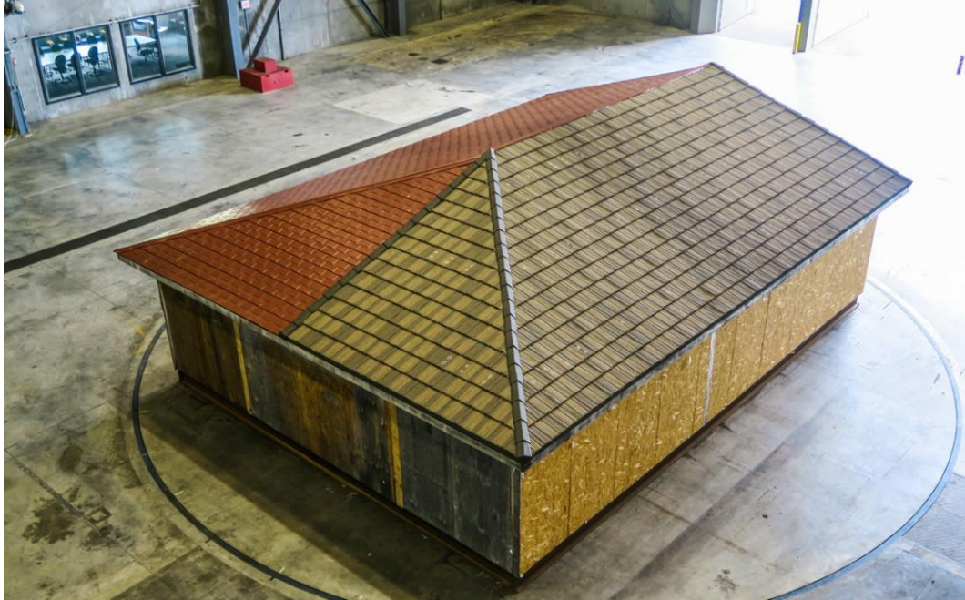
Figure 3.1: Photograph of the test building located in the IBHS test chamber. The two halves of the roof are clad with two different discontinuous metal roofing products.
