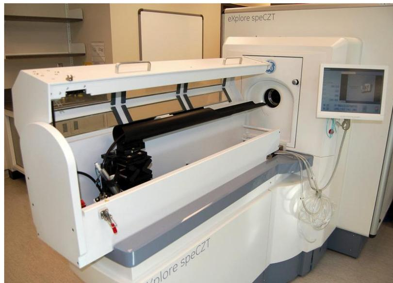
**Figure 2.2: GE eXplore speCZT.** Located at Robarts Research Institute, it is a cone-beam micro-CT imaging system, which we used in this work to characterize diffusion of a contrast-agent drug surrogate (Iohexol).
