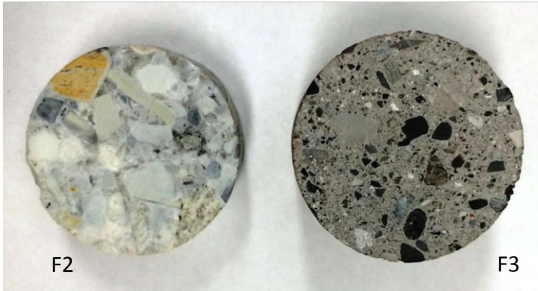
**Figure A.1. Photographic cross sections of F2 and F3 cores. Note the difference in colour, texture and clast populations. F3 is more representative of the particulate impact melt at Haughton. Cross section of each core is approximately 2.5 cm.**
