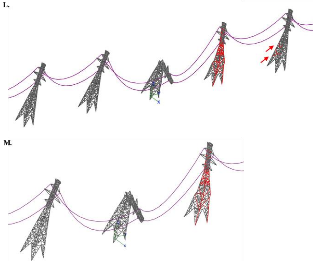
Figure 3-12: Progressive failure of S2 tower in second critical scenario, \lambda = 9.4 . (A) 10%; (B) 12.5%; (C) 15%; (D) 17.5%; (E) 22.5%; (F) 25%; (G) 27.5%; (H) 30%; (I) 32.5%; (J) 35%; (K) 37.5%; and (L,M) 40%.
