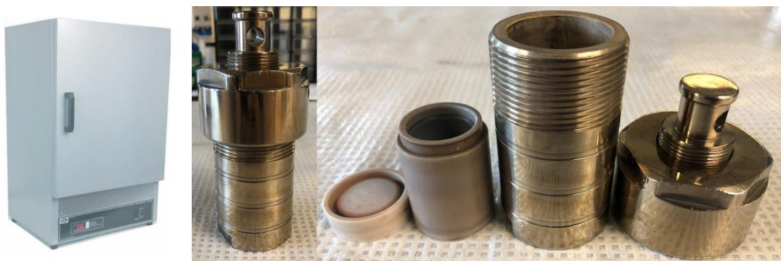
Figure 2.1 Photos of the lab oven and the autoclave for synthesis.
