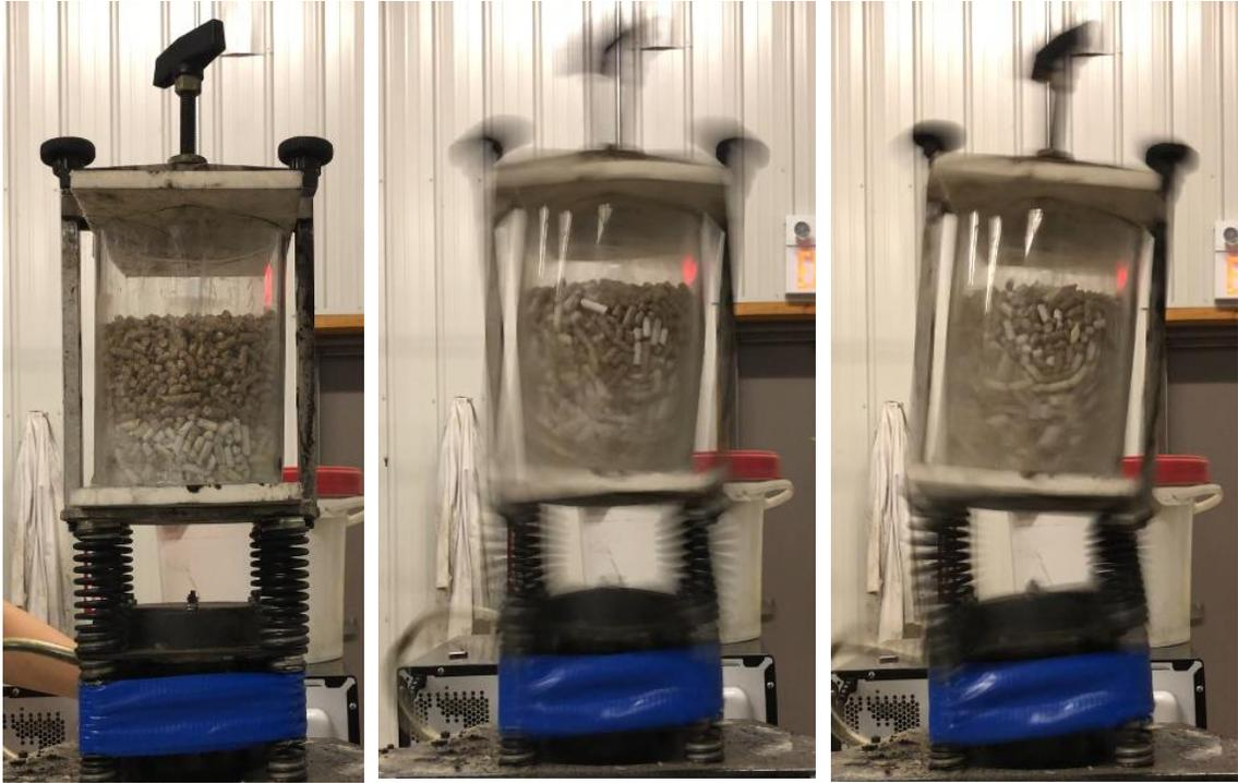
Figure B-1: Still frames of video taken showing PSR mixing capabilities taken at (a) 0 s; (b) 10 s and (c) 30 s.
