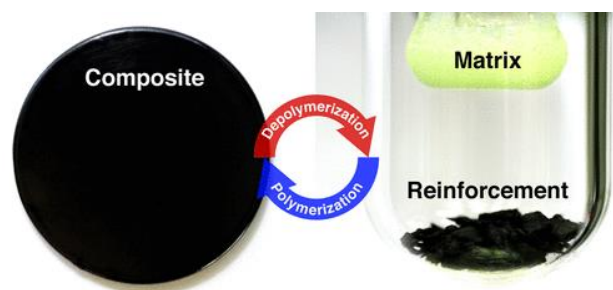
Figure 1.19: Composites composed of carbon fiber and PPA (left) can be fully disintegrated to the starting carbon fiber (right, bottom) and o -PA (right, top) before the reproduction of the composite. Adapted with permission from reference 102. Copyright 2019, American Chemical Society.
