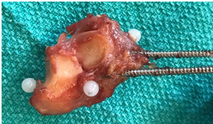
Figure 2.7 Fiducial Markers in Carpal Bone. Fiducial markers placed over prominent carpal bone landmarks for the purpose of digitization and cluster point registration within computational model.
