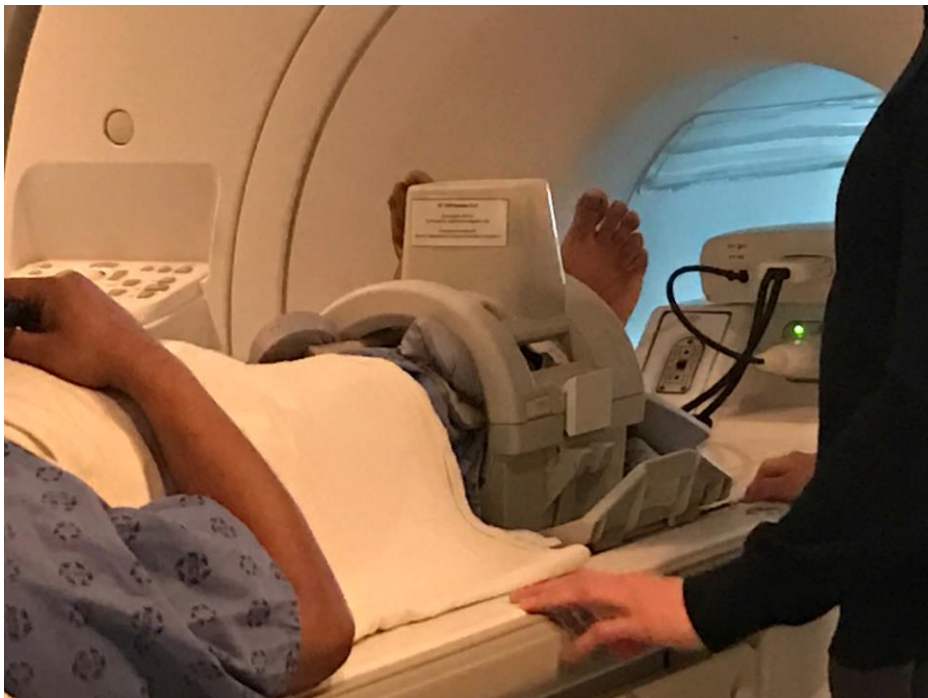
Figure 3-1: Custom-made RF coil and position of the right leg in the MRI.
