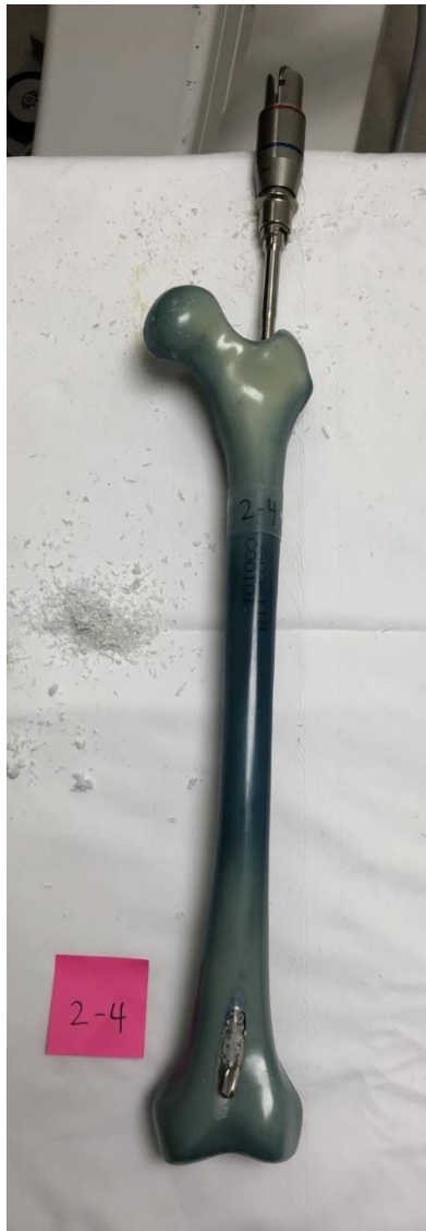
Figure 2.3. Eccentric reaming of the anterior cortex using the 10mm reamer created the anterior cortical perforation of the distal femur. The reamer was advanced further until the full thickness perforation had been created.
