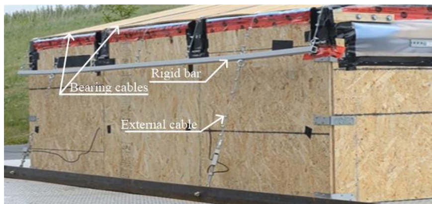
Figure 5.5: Retrofitted control test setup prepared by Rosenkrantz (2017).
