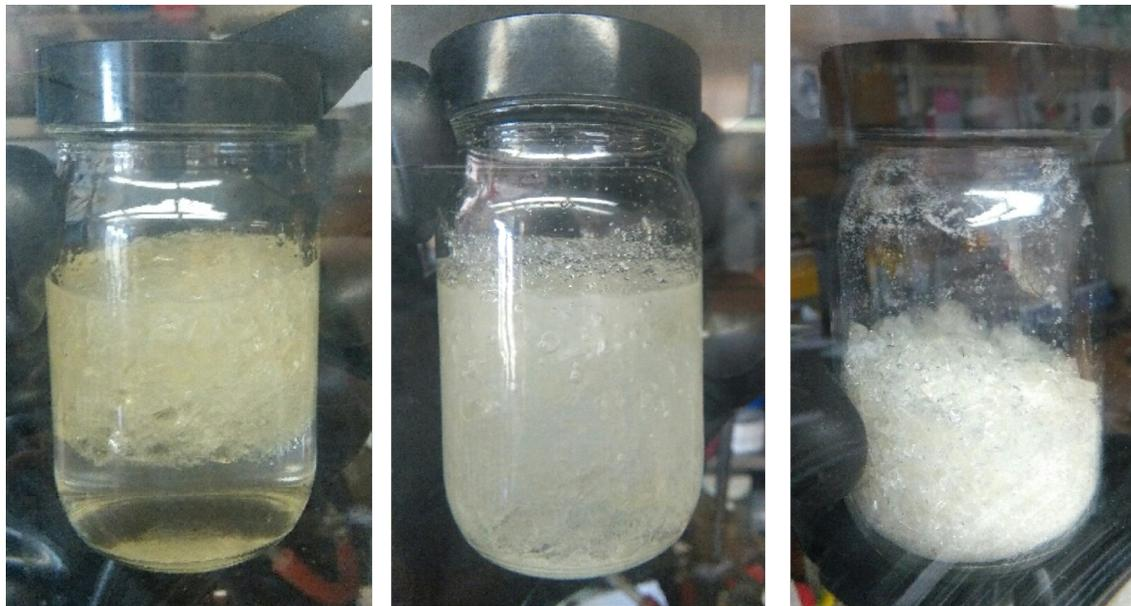
**Figure 7.3:** Demonstration of swellability for network **4.1** in  $\text{CH}_2\text{Cl}_2$  during the leaching process. Notice how the slight yellow colour the crude material disappears after leaching. (A) Initial addition of  $\text{CH}_2\text{Cl}_2$ ; (B) swelled overnight; (C) Dried material after three rounds of leaching.
