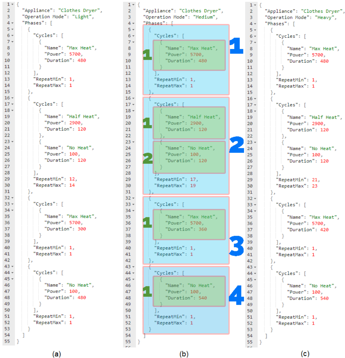
Figure 4.3: SUP representation objects for a clothes dryer, phases are highlighted and numbered in blue, while cycles are in green. Three operation modes are shown (a) Light operation mode. (b) Medium operation mode. (c) Heavy operation mode.
