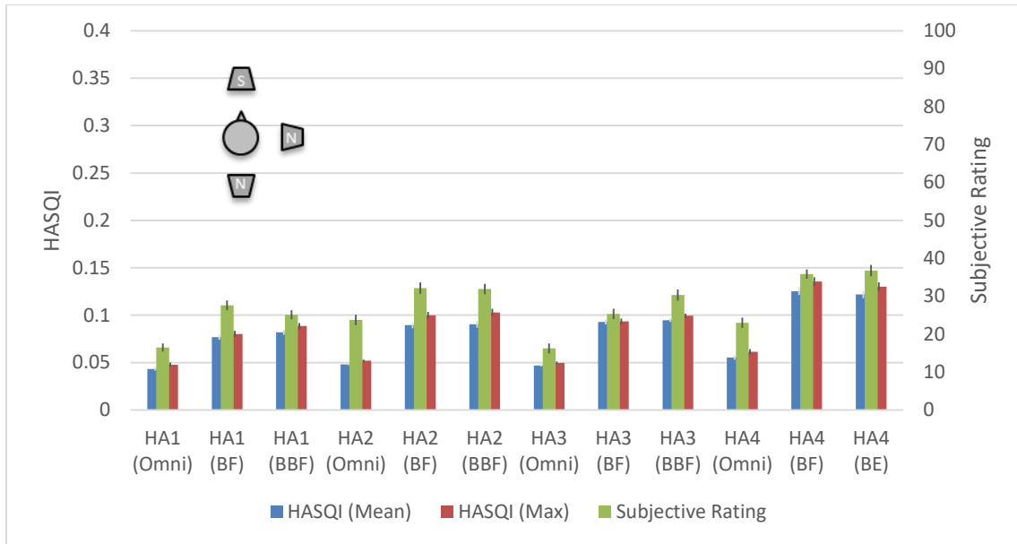
Figure 5.13: Conditionally averaged subjective rating, left-right maximum HASQI score and left-right mean HASQI score of speech in speech-shaped noise at 0 dB SNR, with speech originating from 0° and the noise from 90° and 180° in the reverberation chamber.
