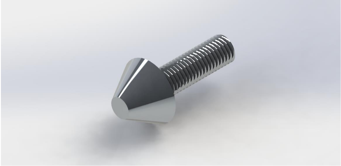
Figure 2.9 The truncated plug used at the hot outlet in the present vortex tube.
