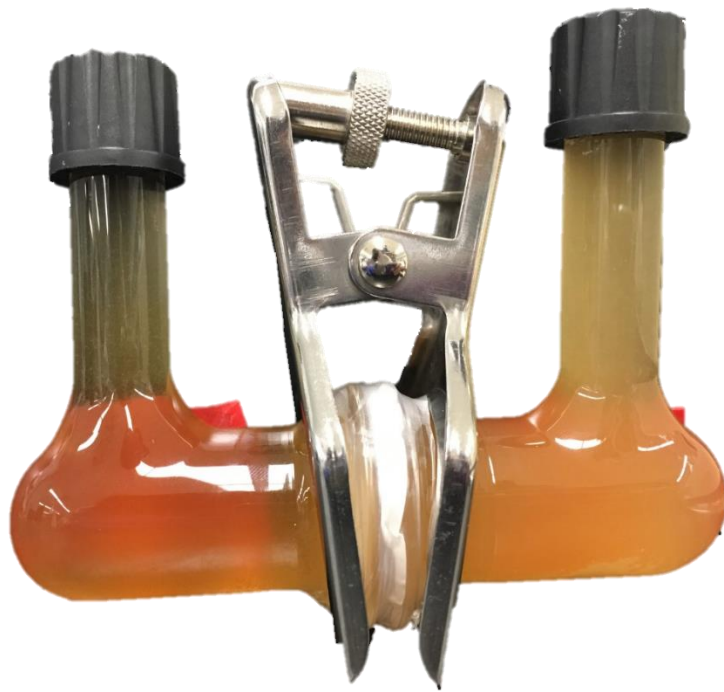
Figure 23. Co-culture apparatus. The apparatus was assembled, sterilized, and filled with VDMP (50mL). Pictured are two chambers clamped together with a 0.45 \mu m filter paper placed between.
