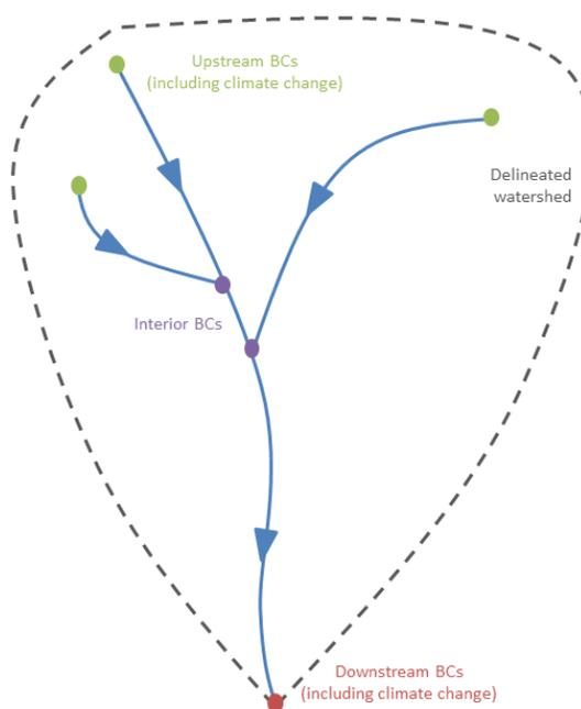
**Figure 22: River schematic identifying locations which require the specification of boundary conditions and where climate change is incorporated into the hydraulic modelling process**
