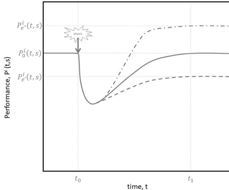
**Figure 3: Conceptual definition of STDRM using system performance graph
