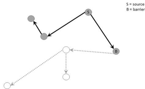
**Figure 66: Conceptual results from a trace downstream operation in a geometric network**
