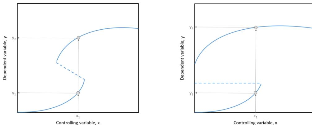
**Figure 7: Four types of threshold responses including (a) no response; (b) step-change; (c) alternate stable state; and (d) irreversible change (adapted from Walker and Salt, 2012)**
