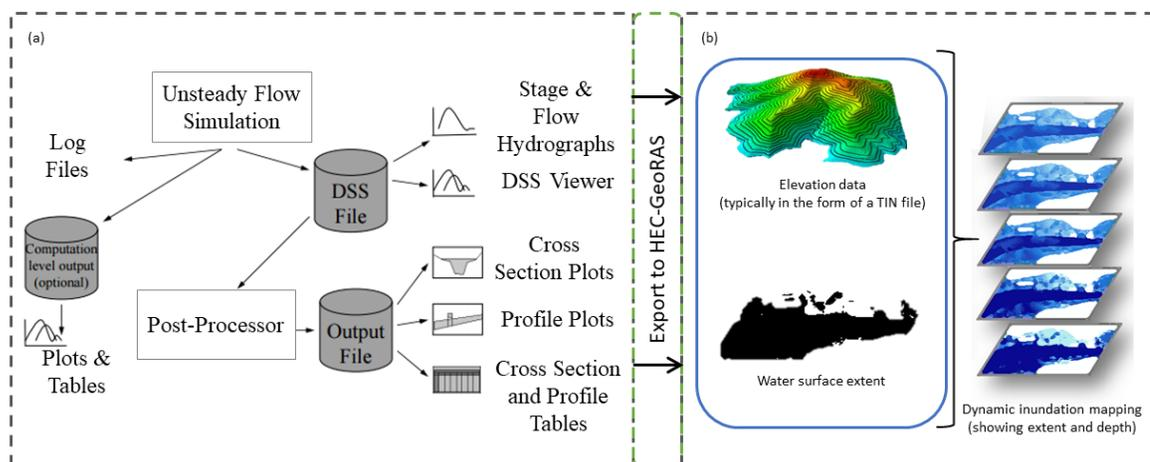
**Figure 23: Schematic of physical domain output (a) generated from hydraulic unsteady flow simulation; (b) when combined with spatial topographical information to generate a time series of inundation maps (adapted from USACE 2010)**
