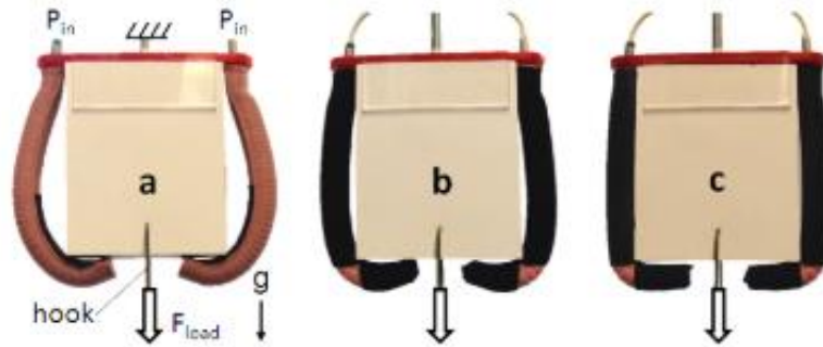
Figure 2.13 Maximum payload test of Fiber Reinforced grippers with different actuator sleeve spacing configurations (Galloway et al. [63], © 2013 IEEE, included with permission).
