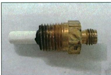
Figure 3.5. Ceramic porous cup attached to Swagelok fittings.
