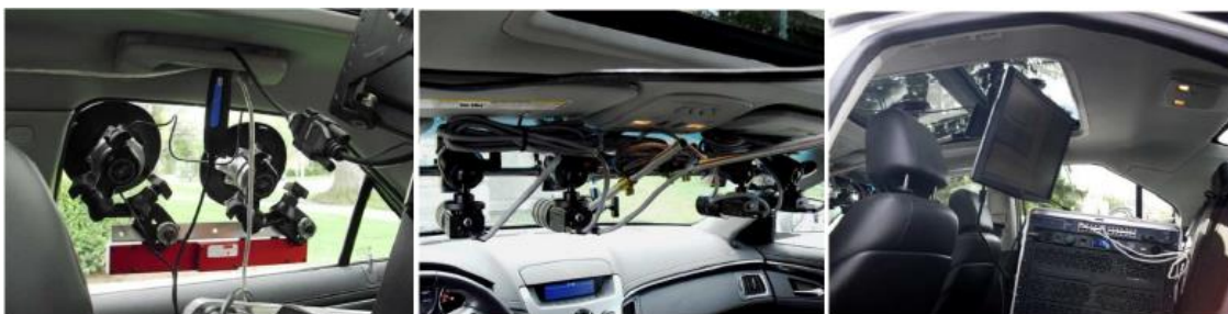
Figure 4. 1 The RoadLab in-vehicle laboratory: a) (left): on-board computer and LCD screen b) (center): dual stereo front visual sensors, c) (right): side stereo visual sensors [4].
