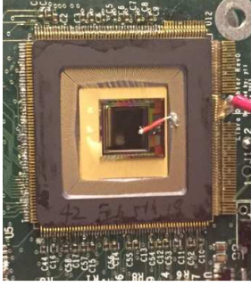
Figure 4.1: Se/CMOS sensor with 7.8\mu\text{m} element size (on the left) has an active area of approximately 1\text{cm}^2 . The CSA model of the micro-sensor array (on the right) includes x-ray interactions, reabsorption, converter blur \tilde{b}(x) , sensor collection efficiency \beta , quanta collection in rectangular apertures \Pi_\epsilon(x) , read-out noise \tilde{n}_\epsilon(x) and discrete sampling \text{III}_\epsilon(x) .
