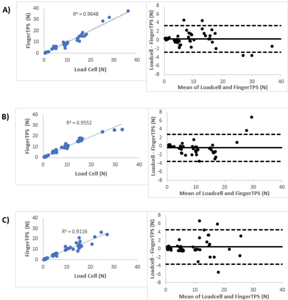
**Figure 2.6** Scatterplot and Bland-Altman plots comparing the measurement of force from the FingerTPS sensors and Loadcell. A linear fit was used to calculate the correlation between the two measurement systems. For the Bland-Altman plots, the solid line represents the average difference, or bias, and the dashed lines indicate the limits of agreement. A) Trial 1, N=50; B) Trial 2, N=50; C) Trial 3, N=41.
