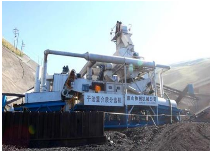
Figure 2.18 The commercial modularized Air Dense Medium Fluidized Bed by Zhao et al.
