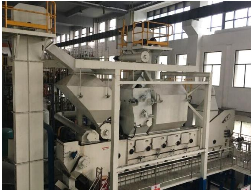
Figure 8.2 A semi-industrial Air Dense Medium Fluidized Bed system for dry coal beneficiation.
