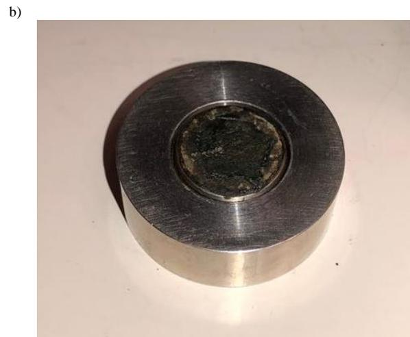
**Figure 1.19:** a) Buehler MicroMet 5100 series device for hardness testing. b) The mounted sample being used for the hardness test using the paraffin wax.
